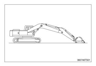
2. Disconnect hoses(A) from rod side of boom cylinder and drain oil from cylinders and hose.(Put cups on piping and hose ends)
