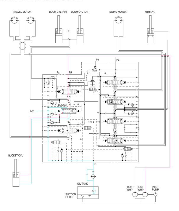
When the right control lever manually is placed in the bucket roll out position.
