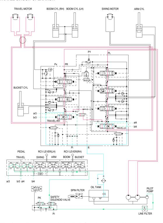
When the travel levers are manually placed to the forward or reverse position.
