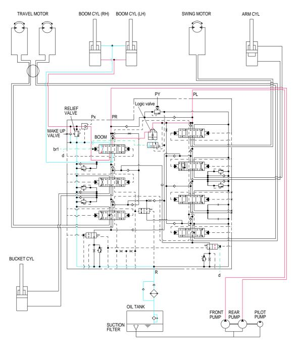
When the right control lever is pulled to boom raise position. Then the oil from pilot pump through the remote control valve to boom sections of the control valve.
