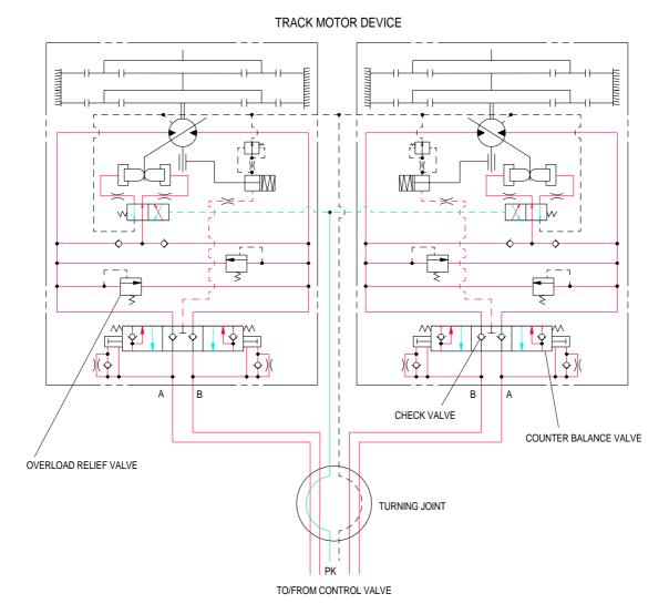
Brake valves are provided on travel motors to offer the following functions.
