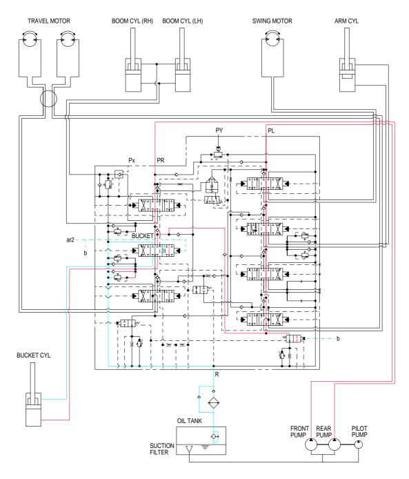
When the right control lever manually is placed in the bucket roll in position.
