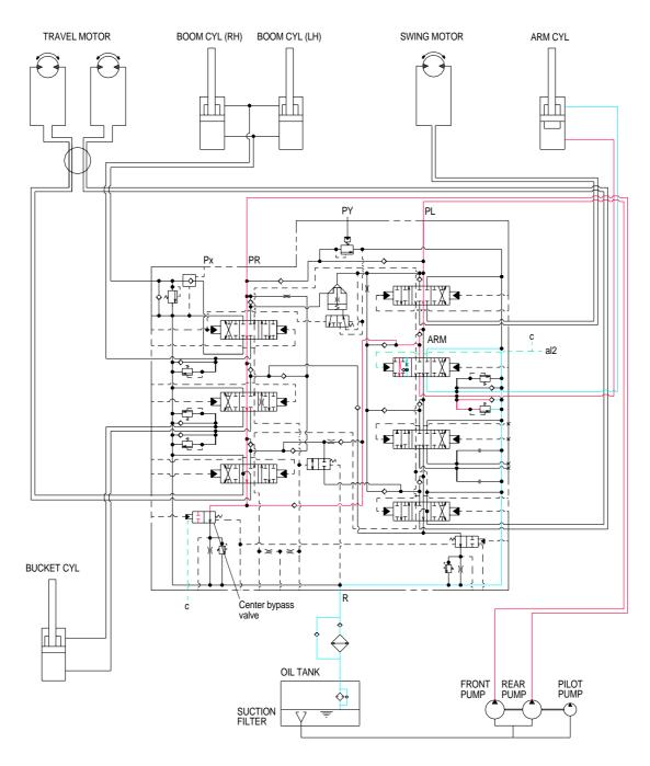
When the left control lever manually is placed in the arm roll in position.
