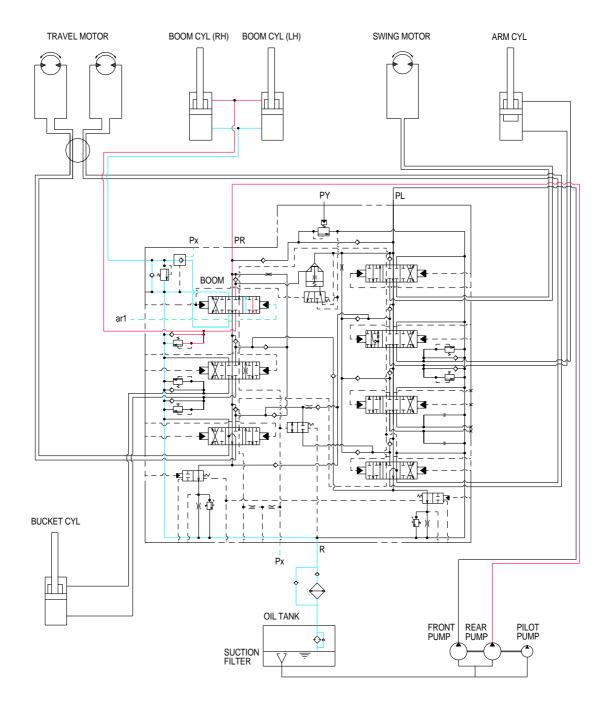
When the right control lever is pushed forward to boom lower position. Then the oil from pilot pump through the remote control valve to boom sections of the control valve. Here, the spool positions are moved to the boom lower position, and the boom lower circuit is opened.
