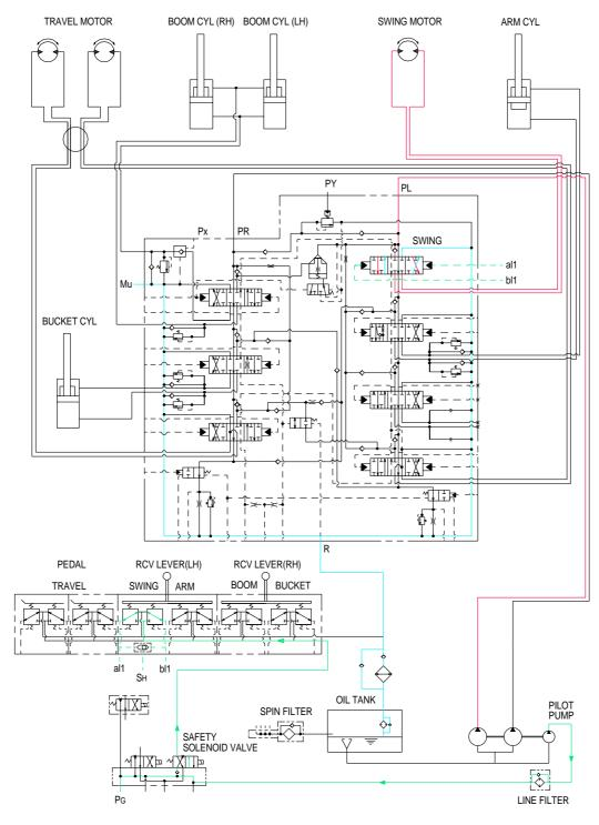
When the left control lever manually is placed in the swing position. Then the oil flows from pilot pump through the pilot valve to the swing section of the control valve. Here, the spool position is moved to right or left swing position.
