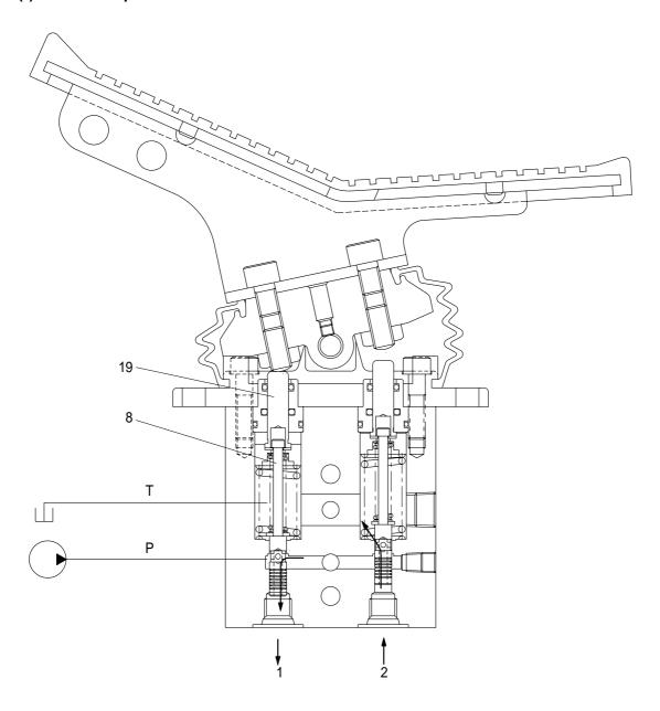
When the push rod(19) is stroked, the spool(8) moves downwards.
