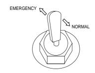
Never place this switch in EMERGENCY position when the CPU is in normal operation.
