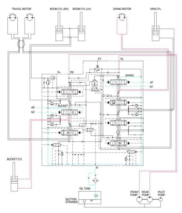
When the swing and bucket functions are operated, the swing and bucket spools changed. The oil flows rear pump through the bucket section of the right control valve to the bucket cylinder and the bucket function. The oil flows from front pump through swing section of the left control valve to the swing motor and swing the superstructure.
