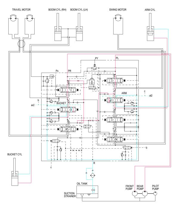
When the bucket in and arm in functions are operated, simultaneously the bucket and arm spools changed.
