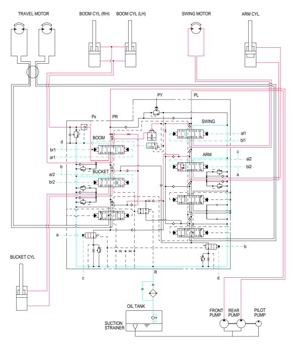
When the swing, boom, arm and bucket functions are operated, the each spools of the control valve changed.
