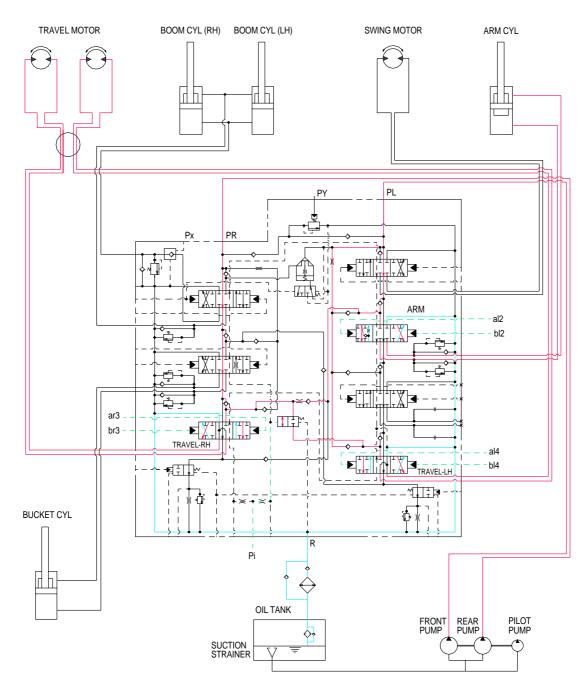
When the arm and travel (RH, LH) functions are operated, the arm and travel (RH, LH) spools and the select valve changed. The oil flows from rear pump through the travel (RH, LH) section of the control valve to the right and left travel motor.
