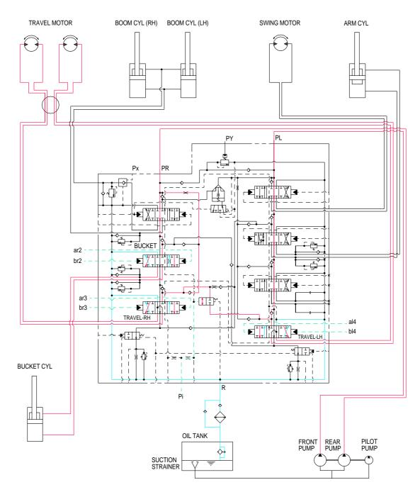
When the bucket and travel (RH, LH) functions are operated, the bucket and travel (RH, LH) spools and the select valve changed. The oil flows from front pump through the travel (RH, LH) section of the control valve to right and left travel motor and the machine traveling.
