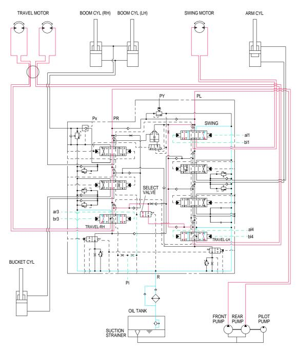
When the swing and right and left travel functions are operated, the swing and travel (RH, LH) spools and the select valve changed. The oil flows from rear pump through the travel (RH, LH) section of the control valve to the right and left travel motor.
