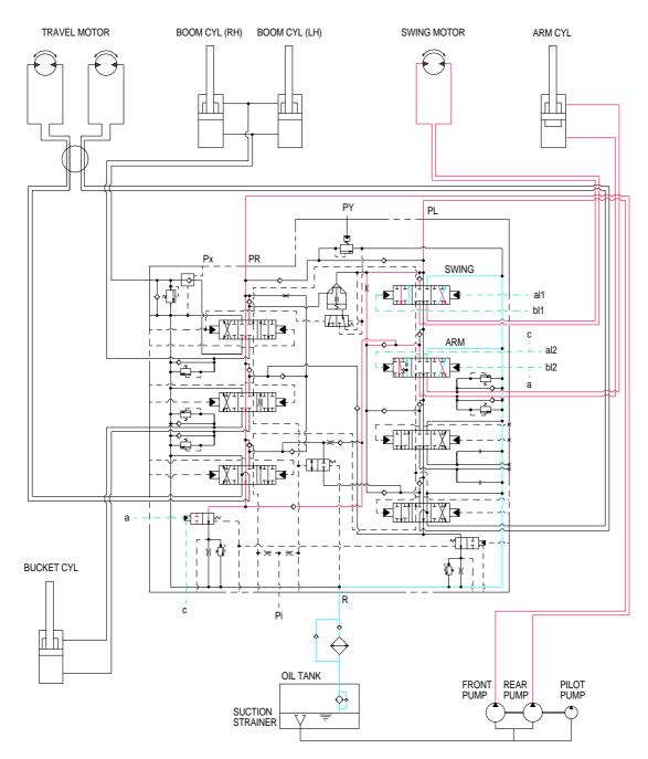
When the swing and arm functions are operated, simultaneously the swing and arm spools changed. The oil flows from the front pump through arm and swing section of the control valve to arm cylinder and swing motor, and the arm and swing function.
