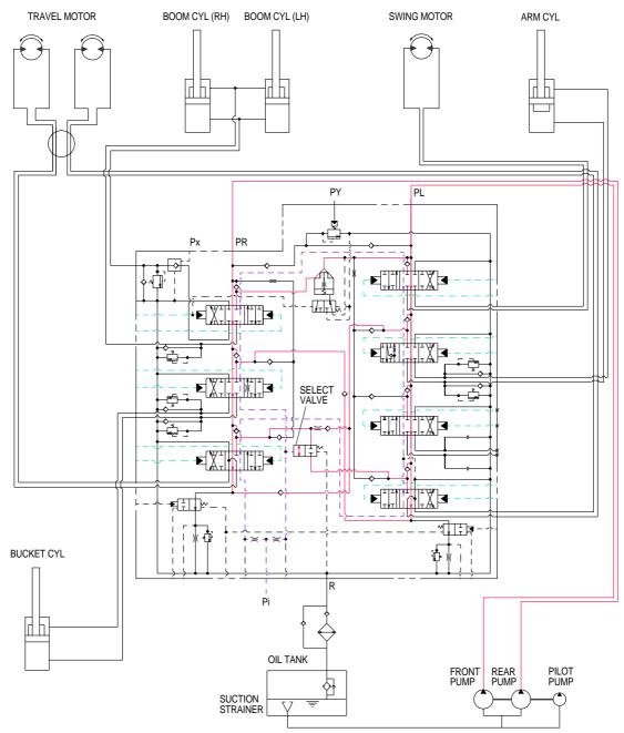
In case operation, the oil flows from both main pumps through the neutral oil passage, bypass oil passage and confluence oil passage. Then the oil is supplied to each actuator and function them. Check valves and orifices are provided with on these flow passage. These control the oil flows from the pump corresponding to the each actuator's state of functioning and smooth the combined operation.
