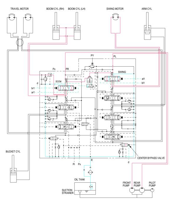
When the swing and boom functions are operated, simultaneously the swing spool and boom spools changed. The oil flows from the rear pump through boom section of the control valve to boom cylinders and the boom functions.
