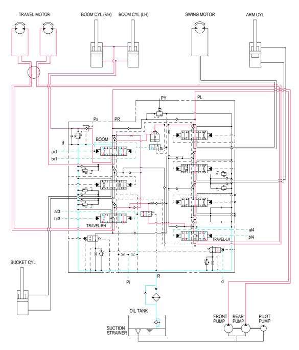
When the boom and travel (RH, LH) functions are operated, the boom and travel (RH, LH) spools and the select valve changed. The oil flows from rear pump through the travel (RH, LH) section of the control valve to the right and left travel motor.
