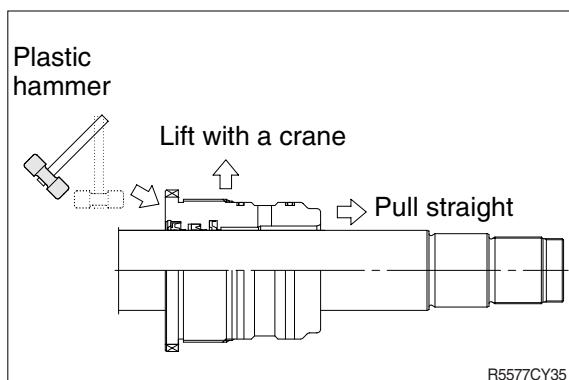
**(3) Disassemble the piston assembly**
