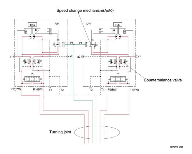
Valves are provided on travel motors to offer the following functions.
