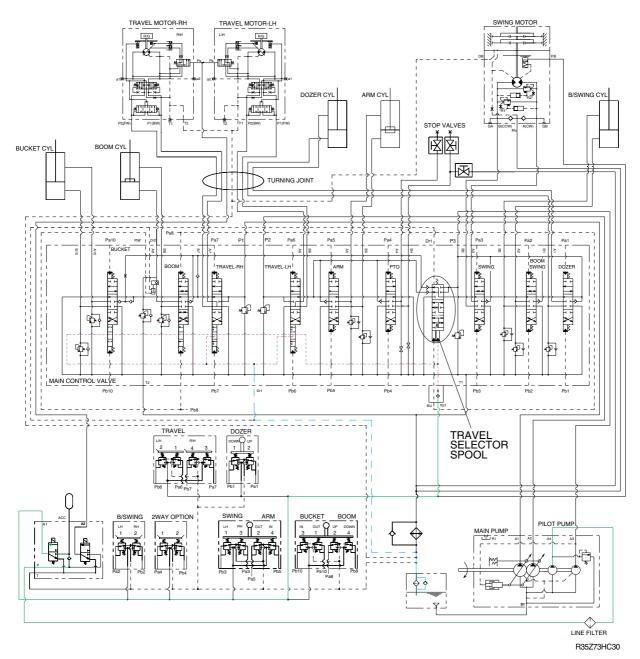
The oil from the P1, P2, P3 pump flows through the neutral oil passage, bypass oil passage and confluence oil passage in the main control valve. Then the oil goes to each actuator and operates them. Check valves and orifices are located on these oil passage in the main control valve. These control the oil from the main pumps so as to correspond to the operation of each actuator and smooth the combined operation.
