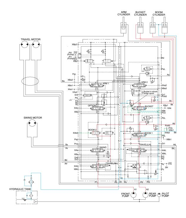
When the boom up and bucket functions are operated, simultaneously each spool in the main control valve is moved to the functional position by the pilot oil pressure from the remote control valve. Also, the boom up operation preference function is operated by the pilot pressure PCk (refer to page 2-33).
