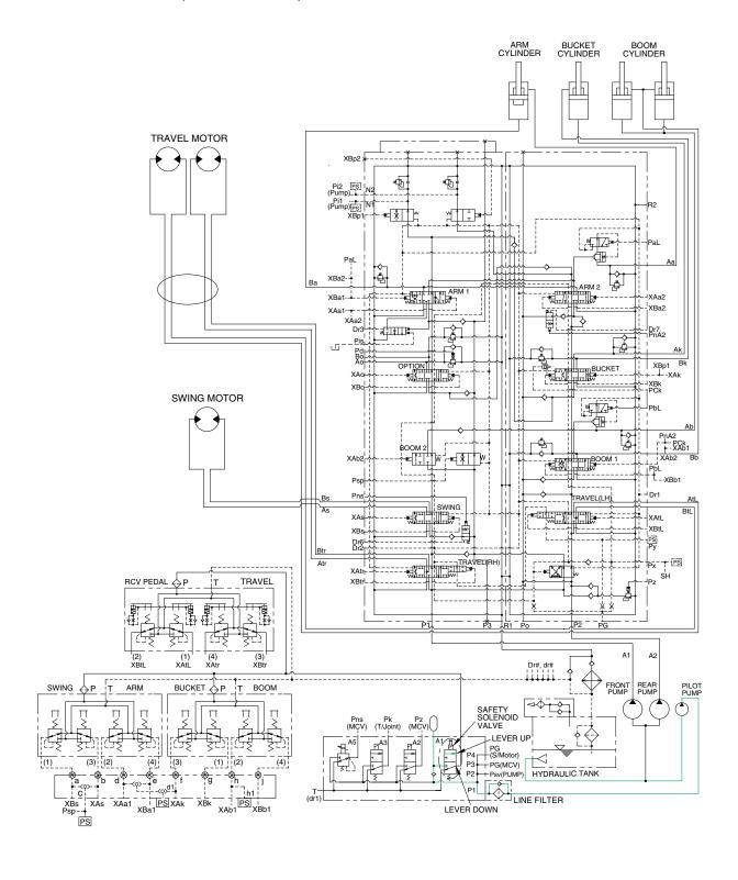
When the lever of the safety solenoid valve is moved upward, oil flows into the remote control valve through solenoid valve and line filter.
