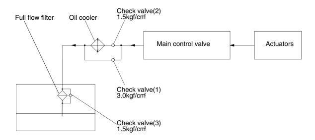
All oil from each actuator returns to the hydraulic tank through the control valve.
