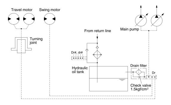
Besides internal leaks from the motors and main pump, the oil for lubrication circulates. These oil have to be fed to the hydraulic tank passing through spin filter and full flow filter in the hydraulic tank. When the drain oil pressure exceed 1.5 kgf/cm² (21psi), the oil returns to the hydraulic tank directly.
