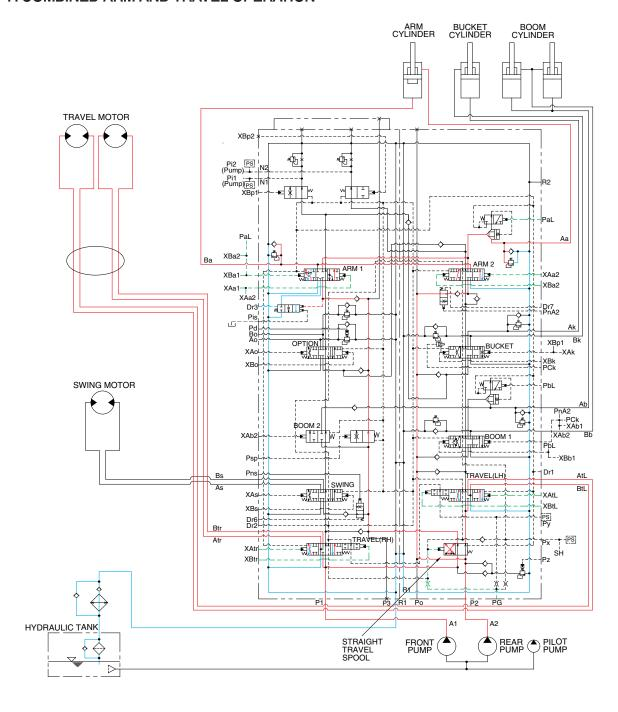
When the arm and travel functions are operated, simultaneously the arm spools and travel spools in the main control valve are moved to the functional position by the pilot oil pressure from the remote control valve and the straight travel spool is pushed to the right by the oil pressure from pilot pump.
