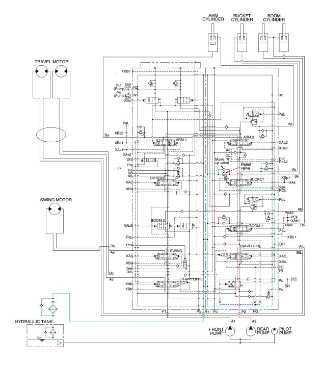
When the right control lever is pushed right, the bucket spool in the main control valve is moved to the roll out position by the pilot oil pressure from the remote control valve.
