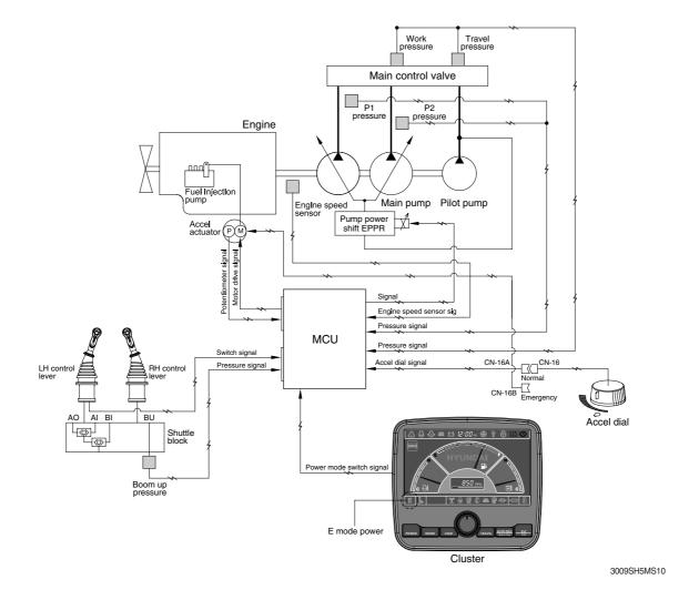
The variable power control system controls the engine and pump mutual power according to RCV lever stroke and pump load.
