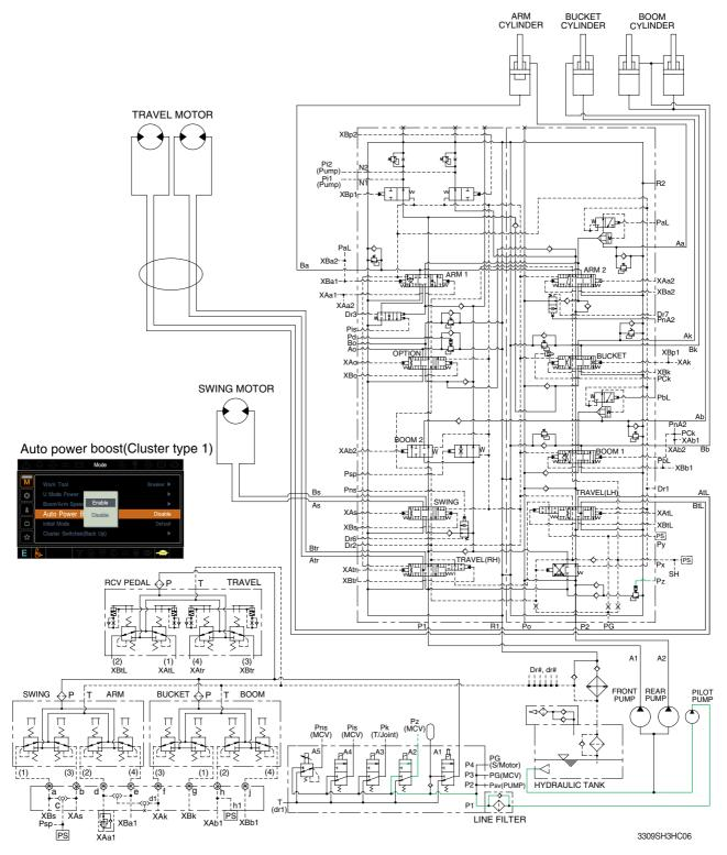
When the power boost switch on the left control lever is pushed ON, the power boost solenoid valve is actuated, the discharged oil from the pilot pump flows into **Pz** port of the main relief valve of main control valve; then the setting pressure of the main relief valve is raised from 350 kgf/cm<sup>2</sup> to 380 kgf/cm<sup>2</sup> for increasing the digging power.
