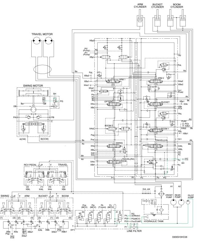
When one of the RCV lever (except travel lever) is tilted, the pilot oil flows into SH port through main control valve.
