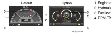
1 Engine coolant temperature gauge
