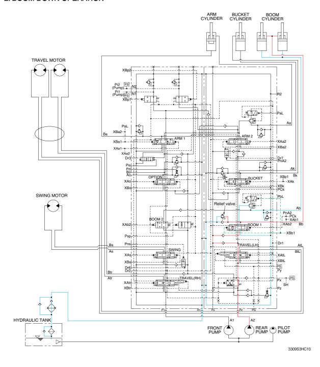
When the right control lever is pushed forward, the boom 1 spools in the main control valve are moved to the down position by the pilot oil pressure from the remote control valve.
