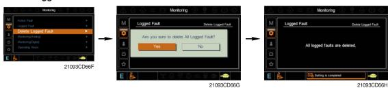
· The logged faults of the MCU can be deleted by this menu.
