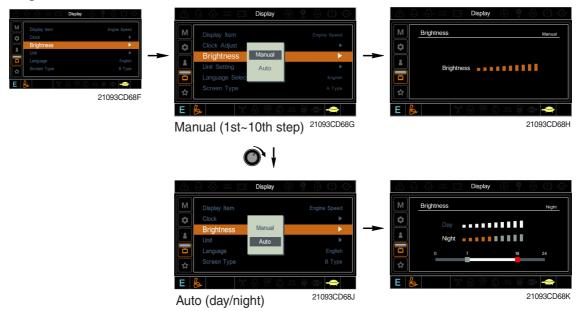
If "Auto" is chosen, brightness for day and night can be differently set up. Also by using the bar in lower side, users can define which time interval belongs to day and night.
