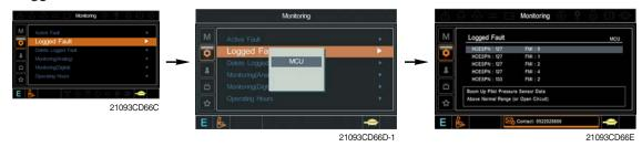
· The logged faults of the MCU can be checked by this menu.
