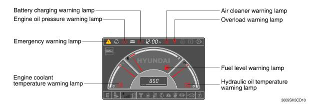
Each warning lamp on the top of the LCD pops up on the center of LCD and the buzzer sounds
