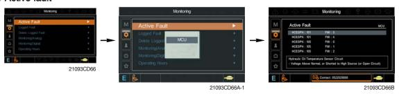
· The active faults of the MCU can be checked by this menu.
