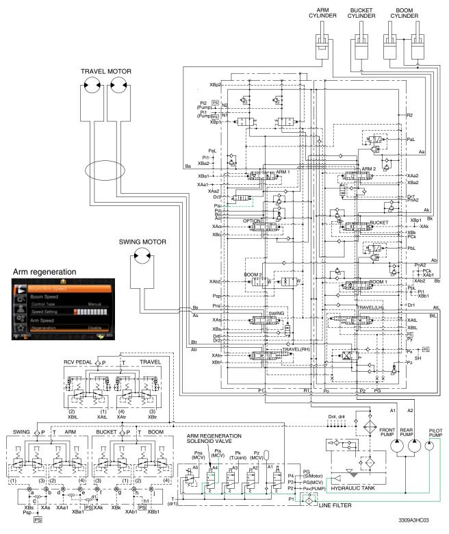
When the arm regeneration is selected to disable on the cluster, the arm regeneration solenoid valve is activated. The pilot oil from pilot pump flow into **Pis** port in main control valve through solenoid valve and the arm regeneration spool is shifted to left.
