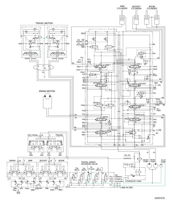
When the travel speed switch is pushed, the travel speed solenoid valve is actuated and the discharged oil from the pilot pump flows to the **P** port of pilot valve in the travel motors.
