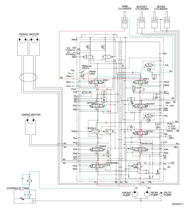
When the left control lever is pulled back, the arm spools in the main control valve are moved to the roll in position by the pilot oil pressure from the remote control valve.
