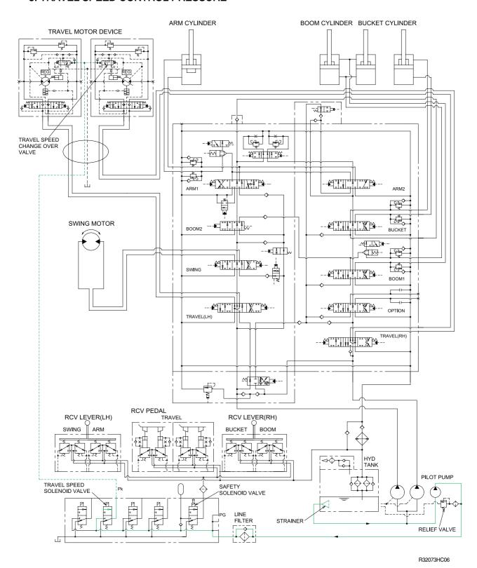
When the travel speed solenoid valve was placed in the Hi position, the pressure oil from pilot pump through line filter flows to port(Pk) of travel speed change over valve, and the control piston is pushed up, thus minimizing the displacement.
