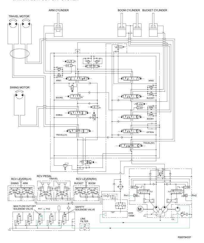
When the breaker operation mode is selected on the cluster, max flow cut off solenoid valve actuates automatically. Thus pilot pressure(Pm1,Pm2) is sent to the regulator and pump discharge volume is decreased.
