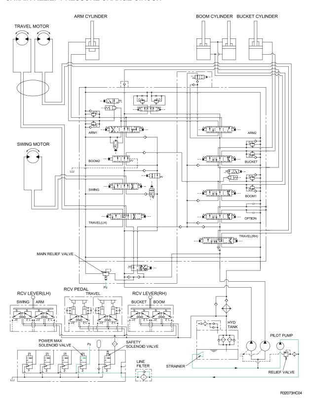
When the power max switch on the left control lever is pushed ON, the power max solenoid valve is actuated, the discharged oil from the pilot pump into Pz port of the main relief valve of main control valve; Then the setting pressure of the main control valve is raises from 330kgf/cm² to 360kgf/cm² for increasing the digging power. And even when press continuously, it is canceled after 8 seconds.
