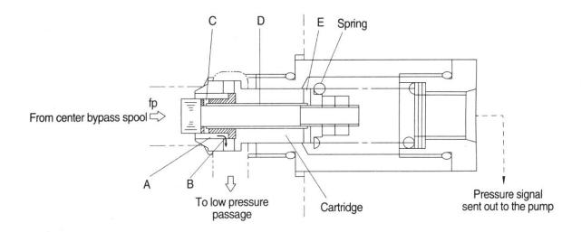
Oil from the center bypass spool valve flows into the tank via passage(A), throttle(B) and the low pressure passage.
