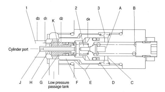
Poppet(F) is securely seated because the cylinder port pressure is normally higher than the tank pressure and  $d_3 < d_4$ .
