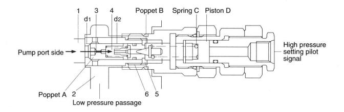
This relief valve is built-in between the pump port side(1) and low pressure passage(2). Hydraulic oil from the pump port side enters chamber(4) via orifice(3) of poppet(A). Because d1<d2, poppet(A) is securely seated.
