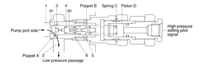
When the above oil flow is formed, pressure drops before and behind orifice(3); when pressure of chamber(1) X area d1 is larger than pressure of chamber(2) X area d2, poppet(A) is lifted and hydraulic oil flows into the low pressure passage.
