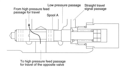
The spool(A) moves to the left; the high pressure passage for travel of the opposite valve( $T_L$ ) and the high pressure passage for travel( $T_R$ ) are connected, and equal amount of oil flows to  $T_R$  and  $T_L$ .
