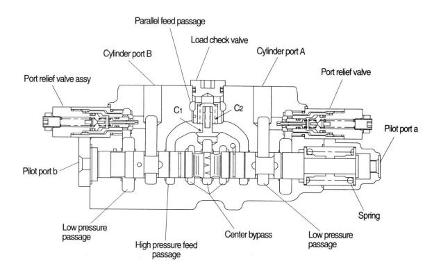
In neutral, spring sets the plunger at the neutral position; the high pressure feed passage is shut off by the plunger; oil from the pump flows through the center bypass.
