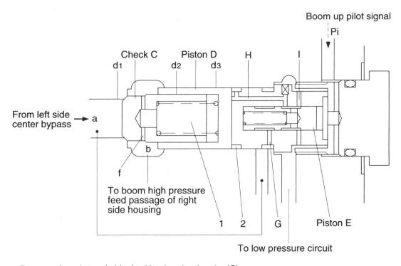
Passage from b to a is blocked by the check valve(C).
