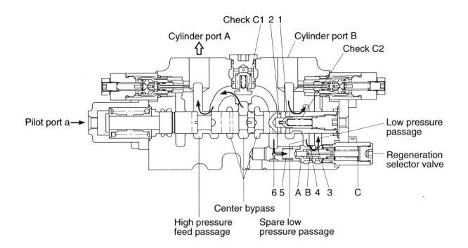
If PP is higher than PB: Return oil from cylinder port B is shut off by check valve(C2) in the plunger and passage(2) is blocked from passage(1). Pressure of high pressure feed passage PP is led into chamber(5) via passage(6). When pressure PP rises higher than the preset pressure of spring(C), piston(A) and spool(B) move to right; passage(3) and passage(4) are connected; return oil from cylinder port B flows into low pressure passage via spare low pressure passage, passage(4) and passage(3).
