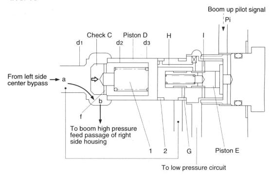
Spring force sets piston(D) at the shown position; check valve(C) is lifted; oil flows through from a to b.
