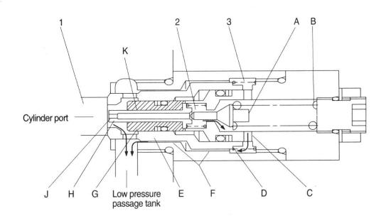
Hydraulic oil from chamber(1) enters chamber(2) via throttle(K) at the tip of poppet(A); it flows around poppet(A) and into the low pressure passage via side hole(C) and passage(E). Pressure drops before and behind throttle(K), making pressure of chamber(1) x area d1>pressure of chamber(2) x area d2; poppet(G) is lifted and hydraulic oil flows into the low pressure passage.
