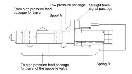
The spring(B) returns the spool(A), which shuts off the high pressure feed passages of TR and TL.
