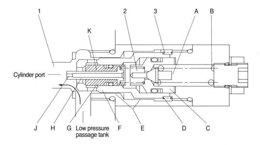
When the cylinder port pressure drops(closer to negative pressure) until the cylinder port pressure is lower than the tank pressure, poppet(F) opens receiving the tank pressure for the difference in area between d<sub>3</sub> and d<sub>4</sub>; oil flows from the tank passage to the cylinder port in order to prevent cavitation.
