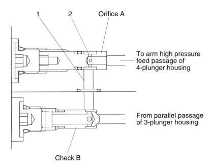
When arm plunger of 4-plunger side is activated, oil from parallel passage of 3-plunger housing pushes up check valve(B); it flows into the high pressure feed passage of the arm plunger via passage(1) and through passage(2) of orifice(A).
