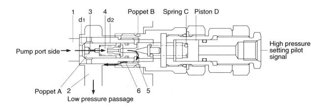
When hydraulic pressure oil reaches the pressure preset by spring(C), pilot poppet(B) opens; oil flows around poppet(B) and into the low pressure passage via side hole(5) and passage(6).
