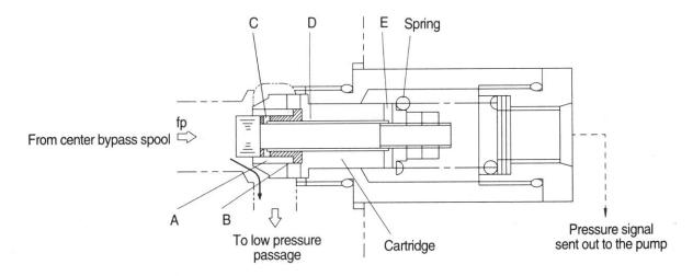
If a large amount flows due to delayed pump response, etc., and pressure fp reaches the preset spring force, then the poppet is lifted and functions as a relief valve.
