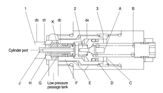
Hydraulic oil from cylinder port enters chamber(2) via orifice(J) of piston(H). Because d1<d2 and d3<d4, poppets(G) and (F) are securely seated.
