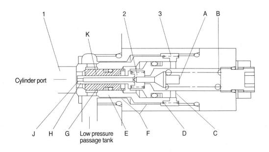
Oil flow is formed; pressure drops before and behind orifice(J); piston(H) moves to right and seats at the tip of poppet(A).
