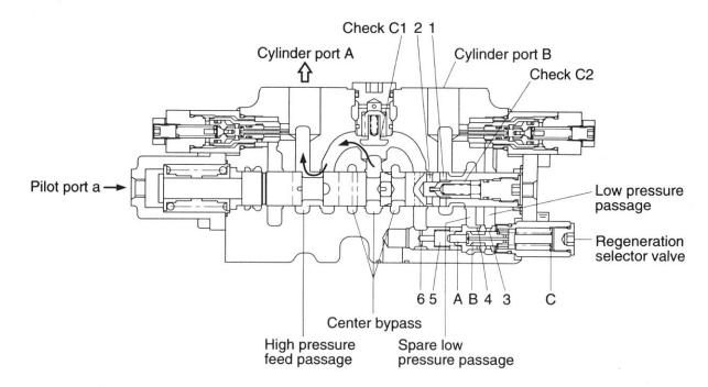
When pressure is applied to pilot port a of the arm plunger, the plunger moves to right as shown; the center bypass passage is shut off; oil from the center bypass pushes up check valve(C<sub>1</sub>) and flows into cylinder port A via the high pressure feed passage.
