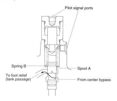
Spring(B) sets spool(A) in position; oil from center bypass flows into the tank passage via the foot relief valve.
