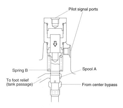
When pilot pressure reaches a preset spring(B) force, the spool(A) moves down and shuts off the flow through the center bypass.
