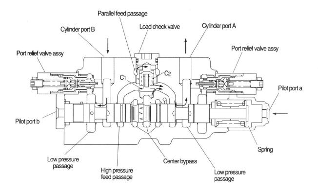
When actuated(pressure is applied to pilot port a), the plunger moves to the left; the center bypass is shut off; oil from the center bypass pushes up the check valve  $C_1$  and flows into cylinder port A via the high pressure feed passage. Meanwhile, oil from the parallel feed passage pushes down check valve  $C_2$  and flows into cylinder port A via the high pressure feed passage.
