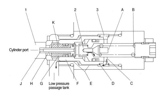
When hydraulic pressure reaches the preset force of spring(B), poppet(A) opens; oil flows around poppet(A) and into the low pressure passage via side hole(C) and passage(E).
