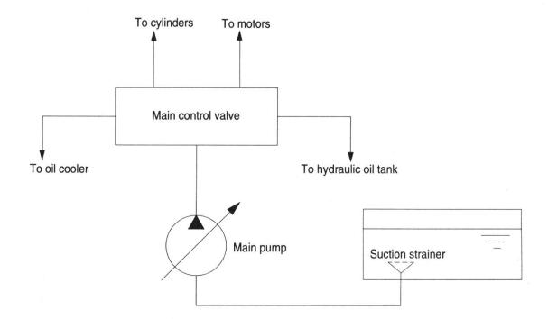
The pump receive oil from the hydraulic tank through a suction strainer. The discharged oil from the pump flows into the control valve and goes out the tank ports.
