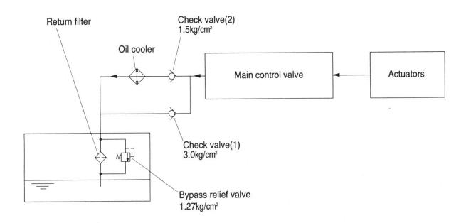
All oil from each actuator returns to the hydraulic tank through the control valve.
