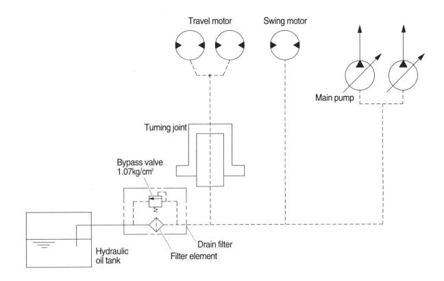
Besides internal leaks from the motors and main pump, the oil for lubrication circulates. These oil have to be fed to the hydraulic tank passing through spin filter.
