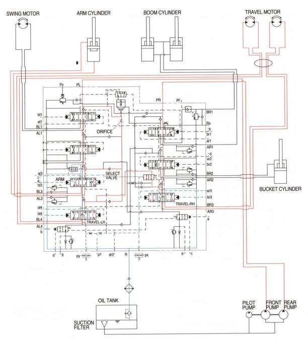
When the arm and travel (RH, LH) functions are operated, the arm and travel (RH, LH) spools and the select valve changed. The oil flows from rear pump through the travel (RH, LH) section of the control valve to the right and left travel motor.
