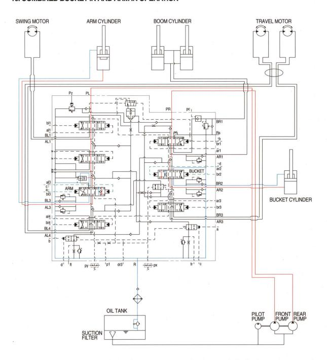
When the bucket in and arm in functions are operated, simultaneously the bucket and arm spools changed.
