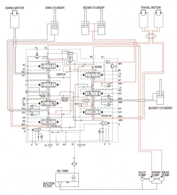
When the boom and travel (RH, LH) functions are operated, the boom and travel (RH, LH) spools and the select valve changed. The oil flows from rear pump through the travel (RH, LH) section of the control valve to the right and left travel motor.
