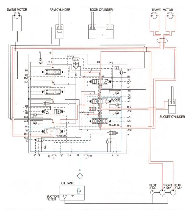
When the bucket and travel (RH, LH) functions are operated, the bucket and travel (RH, LH) spools and the select valve changed. The oil flows from front pump through the travel (RH, LH) section of the control valve to right and left travel motor and the machine traveling.
