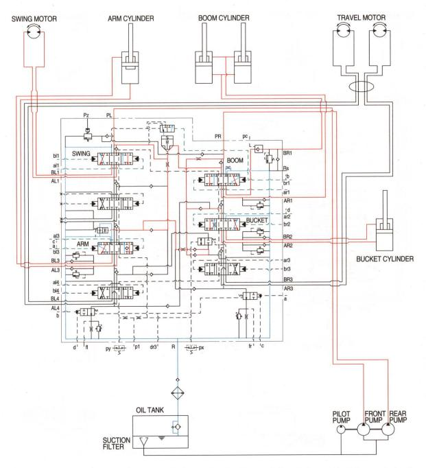
When the swing, boom, arm and bucket functions are operated, the each spools of the control valve changed.
