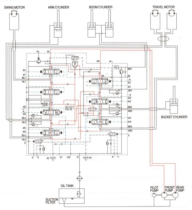
In case operation, the oil flows from both main pumps through the neutral oil passage, bypass oil passage and confluence oil passage. Then the oil is supplied to each actuator and function them. Check valves and orifices are provided with on these flow passage. These control the oil flows from the pump corresponding to the each actuator's state of functioning and smooth the combined operation.
