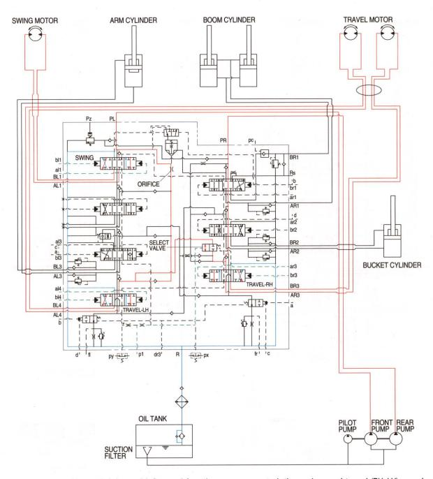
When the swing and right and left travel functions are operated, the swing and travel (RH, LH) spools and the select valve changed. The oil flows from rear pump through the travel (RH, LH) section of the control valve to the right and left travel motor.
