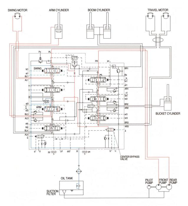
When the swing and arm functions are operated, simultaneously the swing and arm spools changed. The oil flows from the front pump through arm and swing section of the control valve to arm cylinder and swing motor, and the arm and swing function.
