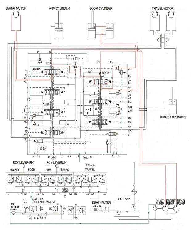
When the swing and boom functions are operated, simultaneously the swing spool and boom spools changed. The oil flows from the rear pump through boom section of the control valve to boom cylinders and the boom functions.
