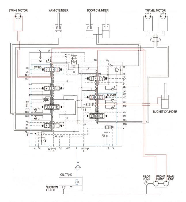
When the swing and bucket functions are operated, the swing and bucket spools changed. The oil flows rear pump through the bucket section of the right control valve to the bucket cylinder and the bucket function. The oil flows from front pump through swing section of the left control valve to the swing motor and swing the superstructure.
