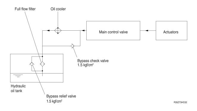
All oil returned from each actuator returns to the hydraulic tank through the main control valve.
