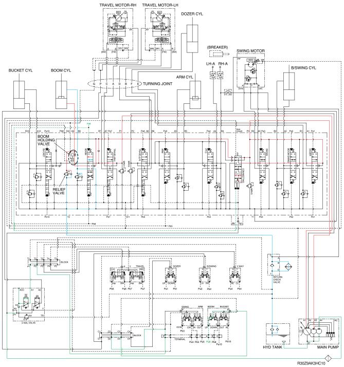
When the right control lever is pulled back, the boom spool in the main control valve is moved to the up position by the pilot oil pressure from the remote control valve.
