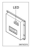
(1) To match the engine torque with the pump absorption torque, CPU controller varies EPPR valve output pressure, which control pump discharge amount whenever feedbacked engine speed drops under the reference rpm of each mode set.
