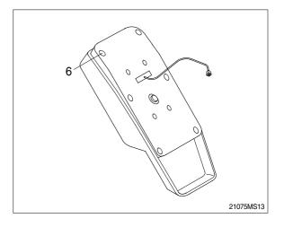
6) Install the new ROM.(Be careful of direction and assmelbe the cluster in the reverse order to removal).
