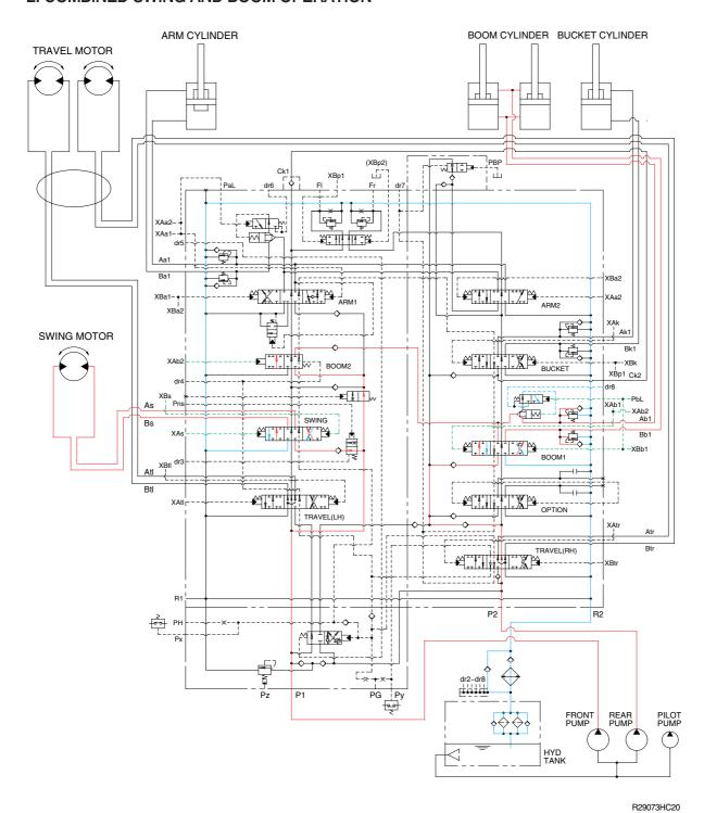
When the swing and boom functions are operated, simultaneously the swing spool and boom spools changed. The oil flows from the rear pump through boom1 section of the main control valve to boom cylinders and the boom functions.
