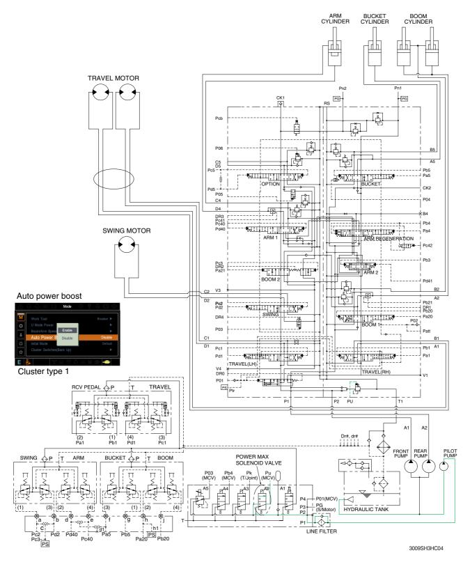
When the power max switch on the left control lever is pushed ON, the power max solenoid valve is actuated, the discharged oil from the pilot pump into Pu port of the main relief valve of main control valve; Then the setting pressure of the main control valve is raises from 350 kgf/cm<sup>2</sup> to 380 kgf/cm<sup>2</sup> for increasing the digging power. And even when press continuously, it is canceled after 8 seconds.
