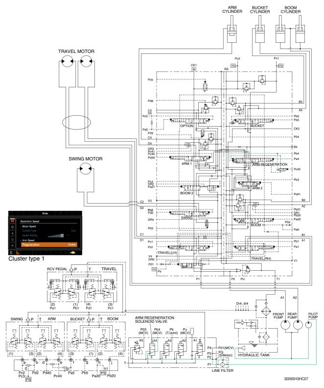
When the arm regeneration is selected to disable on the cluster, the arm regeneration solenoid valve is activated. The pilot oil from pilot pump flow into **Pb4** port in main control valve through solenoid valve and the arm regeneration spool is shifted to right.
