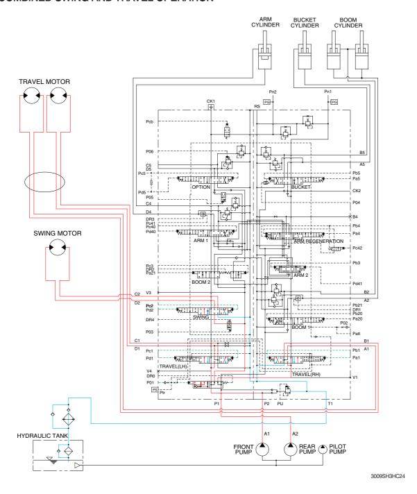
When the swing and travel functions are operated, simultaneously the swing spool and travel spools in the main control valve are moved to the functional position by the pilot oil pressure from the remote control valve. At the same time, the straight travel spool is pushed to the right by the pilot oil pressure from the pilot pump.
