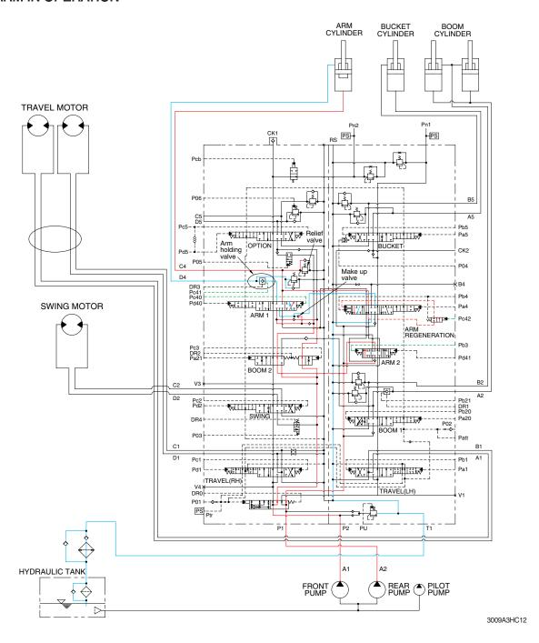
When the LH control lever is pulled back, the arm spools in the main control valve are moved to the roll in position by the pilot oil pressure from the remote control valve.
