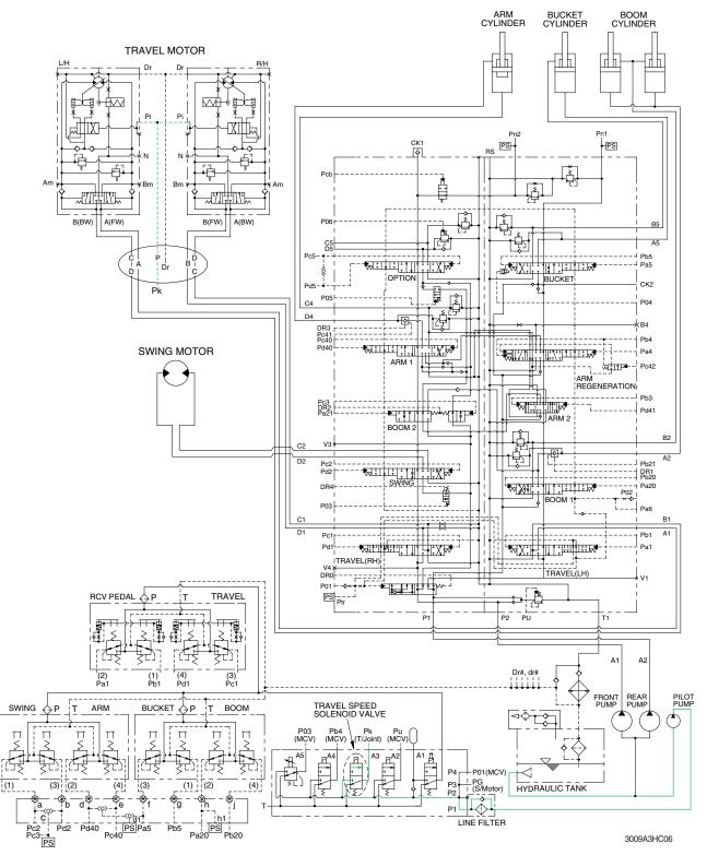
When the travel speed solenoid valve was placed in the Hi position, the pressure oil from pilot pump through line filter flows to port **Pi** of travel speed change over valve, and the control piston is pushed up, thus minimizing the displacement.
