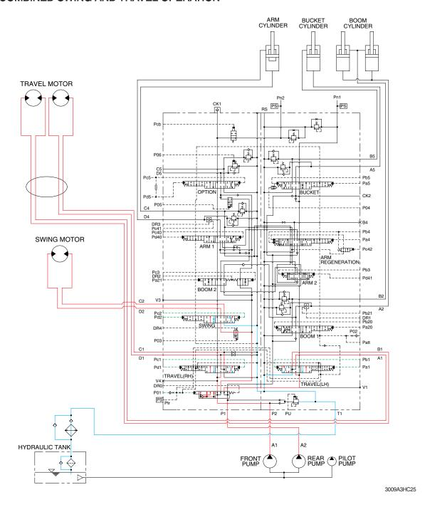
When the swing and travel functions are operated, simultaneously the swing spool and travel spools in the main control valve are moved to the functional position by the pilot oil pressure from the remote control valve. At the same time, the straight travel spool is pushed to the right by the pilot oil pressure from the pilot pump.
