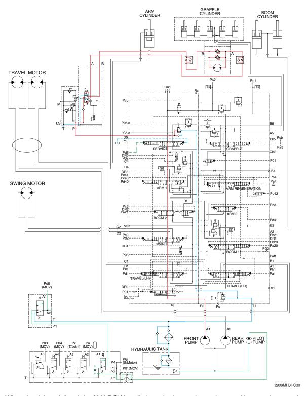
When the right or left switch of LH RCV handle is pushed, grapple rotation spool is moved to grapple clockwise or counterclockwise rotation position by voltage signal engaged to a coil of grapple rotation spool. In both case of grapple clockwise or counterclockwise rotation, voltage signal is engaged to a solenoid valve, then the pilot pressure pushes the service spool in the main control valve right side through Pd5. It leads the oil supply from A1 pump goes to P in the auxiliary valve.
