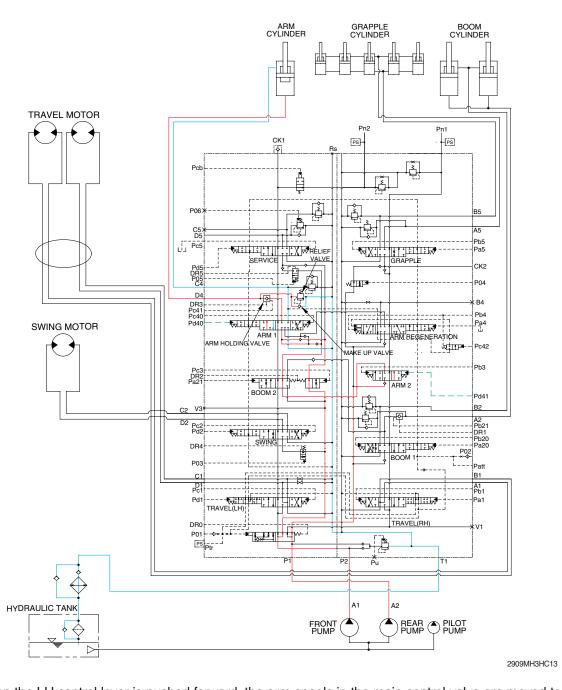
When the LH control lever is pushed forward, the arm spools in the main control valve are moved to the roll out position by the pilot oil pressure from the remote control valve.
