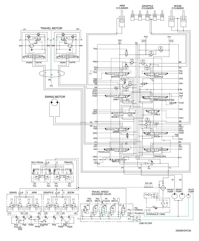
When the travel speed solenoid valve was placed in the Hi position, the pressure oil from pilot pump through line filter flows to port **P** of travel speed change over valve, and the control piston is pushed up, thus minimizing the displacement.
