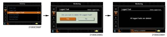
• The logged faults of the MCU or engine ECM can be deleted by this menu.
