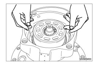
(13) Reassemble brake piston(702) to the casing(301).
