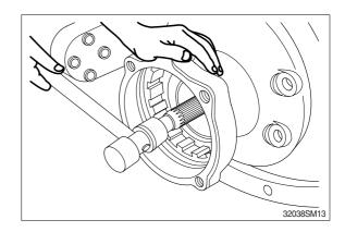
(14) Remove the shoe plate(124) from casing (301).
