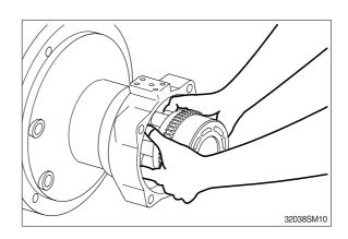
(11) Remove friction plate(742) and separate plate(743) from casing(301).
