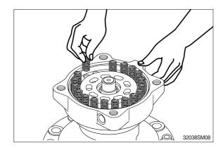
(9) Remove brake piston(702) from casing (301).
