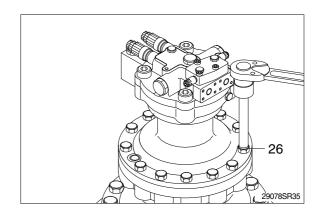
(15) Assemble pressure plug(29), gauge bar(18) and gauge pipe(19).
