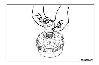
(9) Install the piston sub-assembly(121, 122) to the set plate(123).
