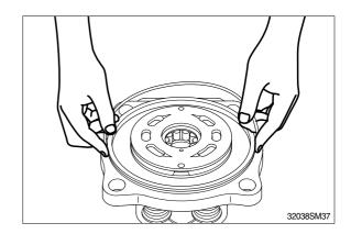
(17) Connect the valve casing(303) with the casing(301) and tighten the hexagon screw(401).
