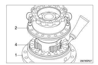
(7) Tighten socket bolts(25) around the middle casing(2).
