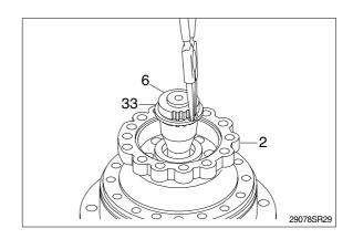
(9) Apply loctite to the tapped holes of the middle casing(2) and then assemble ring gear1(7).
