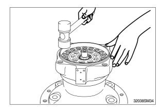
(14) Reassemble brake spring(712) to the brake piston(702).
