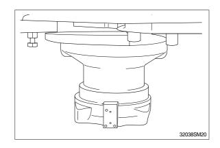
(2) When reassembling the roller bearing, install the snap ring(432), and spacer(106) to the drive shaft(101). Insert the collar and cone of the roller bearing(443). Install the spacer(106) and stop ring(432). Install stop ring(433) to the output shaft (101) by heating the cone of the roller bearing(444).
