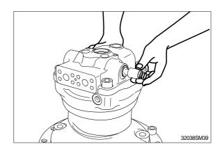
(19) Insert O-rings(051-1) to the relief valve (051) and reassemble them to valve casing(303).
