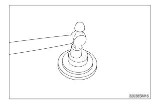
③ Remove the roller bearing(444) from the valve casing(303) by using slide hammer bearing puller.
