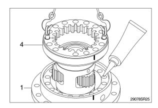
(5) Hammer 4 knock pins(21) around the front casing(1).
