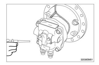
(2) Loosen the drain plug to discharge oil in the casing(301).
