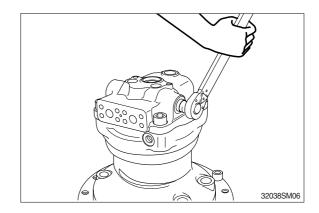
(7) Remove valve casing(303) from casing (301). Then, remove the valve plate(131) from valve casing(303) with care.
