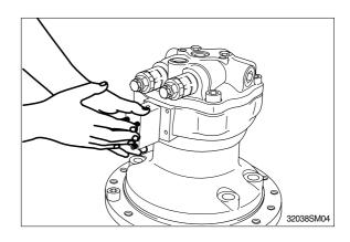
(5) Remove the relief valve(051) from valve casing(303).
