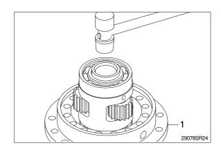
(4) Apply loctite to the front casing(1) and then coincide the matching mark and assemble ring gear2(4).
