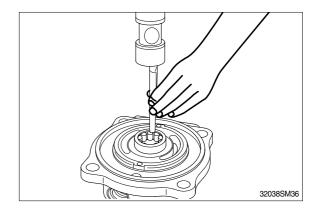
(16) Reassemble valve plate(131) to the valve casing(303) and reassemble O-ring(472).
