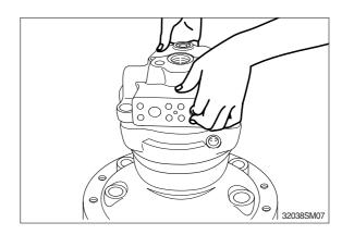
(8) Remove the brake spring(712) from brake piston(702).
