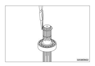
(3) Insert the drive shaft(101) into the casing (301) with the end of output shaft upward and tap the outer race of roller bearing with the hammer.
