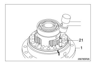
(6) Apply loctite to the ring gear2(4) and then mount middle casing(2) on the front casing(1).
