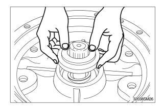
(6) Install the snap ring(437) to the casing (301).
