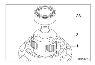
(12) Tighten three M12 eye bolts to drive shaft (3) and remove drive shaft(3) as subassembly.
