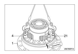
(11) Using the bearing disassembly tool, remove roller bearing(23).
