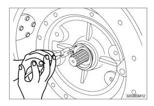
(13) Remove drive shaft(101) from casing (301).
