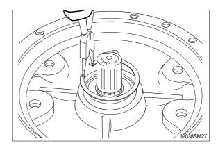
(7) Insert the shoe plate(124) with the casing (301) position horizontally.
