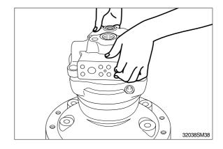
(18) Insert plunger(351) and spring(355) in the valve casing and install O-ring(488). Tighten plug(469) to the valve casing.
