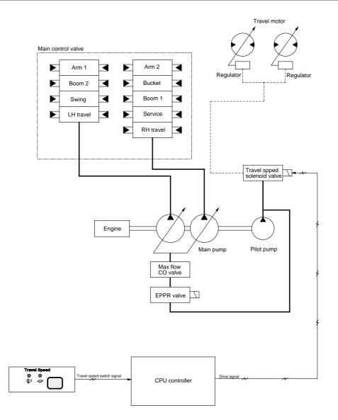
Travel speed can be switched manually by pressing the travel speed switch on the cluster.
