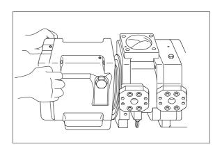
(7) Pull cylinder(141) out of pump casing (271) straightly over drive shaft(111). Pull out also pistons(151), set plate(153), spherical bush(156) and cylinder springs (157) simultaneously.
