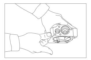
(13) Install cover(C, 629) fitted with adjusting screws(628, 925), adjusting ring(C, 627), lock nut(630), hexagon nut(801) and adjusting screw(924).
