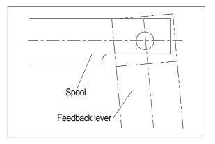
(5) Fit feedback lever(611), matching its pin hole with pin hole in spool. Then insert pin(874). Insert pin in feedback lever a little to ease operation. Take care not to mistake direction of feedback lever.
