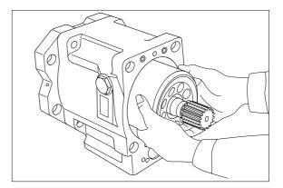
(8) Fit valve plate(313) to valve block(312), entering pin into pin hole. Take care not to mistake suction / delivery directions of valve plate.
