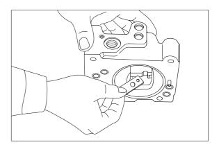
(10) Draw out pin(874) and remove feedback lever(611).
