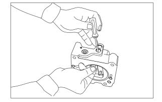
(8) Fit fulcrum plug(614) so that pin forcefitted in fulcrum plug(614) can be put into pin hole of lever(2). Then fix locking ring(858).
