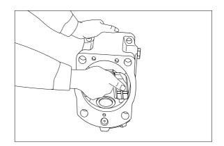
(12) Tapping lightly shaft's end of drive shafts(111, 113) with plastic hammer, take out drive shafts from swash plate supports.
