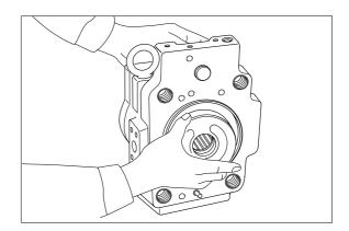
(8) Fit valve block(312) to pump casing (271) and tighten hexagon socket head bolts(401).
