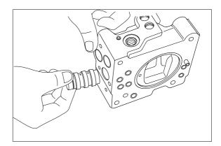
(12) Put spring seat(644), pilot spring(646) and adjusting ring(Q, 645) into pilot hole.Then fix spring seat(624), inner spring(626) and outer spring(625) into compensating hole.
