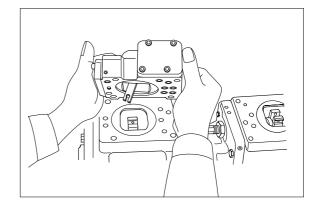
(4) Remove hexagon socket head screw (438) and remove cover(C,629).
