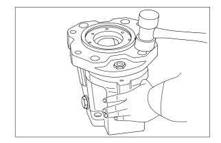
(3) Place pump casing with its regulator fitting surface down, fit tilting bush of swash plate to tilting pin(531), and fit swash plate (212) to swash plate support(251) correctly.
