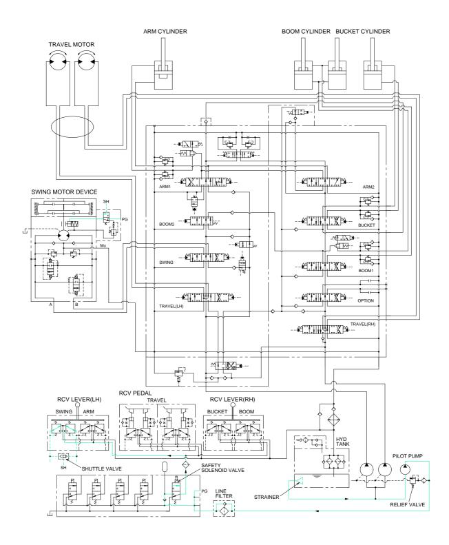
When the swing control lever is operated, the pilot oil flows to SH port of shuttle valve, this pressure move spool so, discharged oil from pilot pump flows to PG port.
