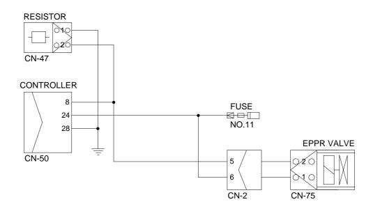
(1) **Test 2:** Check resistance at connector CN-75.
