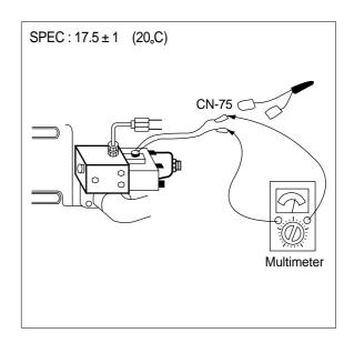
(2) **Test 3**: Check electric current at EPPR valve.
