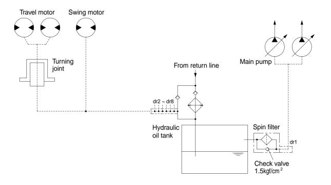
Besides internal leaks from the motors and main pump, the oil for lubrication circulates. These oil have to be fed to the hydraulic tank passing through spin filter and full flow filter in the hydraulic tank. When the drain oil pressure exceed 1.5kgf/cm²(21psi), the oil returns to the hydraulic tank directly.
