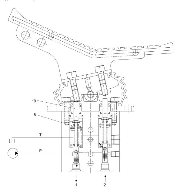
When the push rod(212) is stroked, the spool(201) moves downwards.
