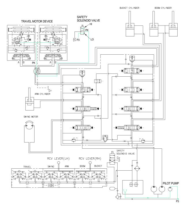
When the travel speed solenoid valve was placed in the HI position, the pressure oil from pilot pump flows to  $P\kappa$  port of 2 speed change over valve, and the control piston is pushed up, thus minimizing the displacement.
