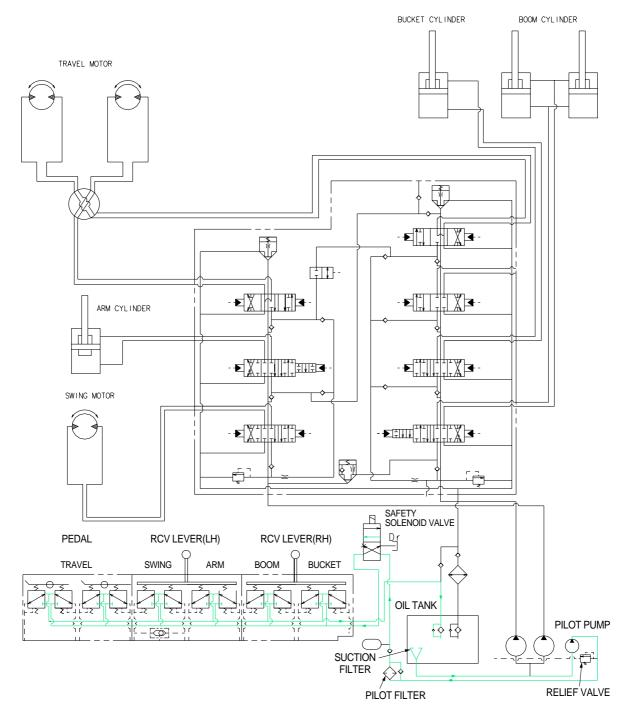
The pilot pump receive oil from the hydraulic tank. The discharged oil from the pilot pump flows to the safety solenoid valve through the pilot filter. The oil is filtered by the pilot filter. The pilot relief valve is provided in the pilot pump for limiting the pilot circuit pressure.
