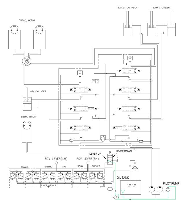
When the lever of the safety solenoid valve moved downward, oil flow remote control valve through solenoid valve and pilot filter.
