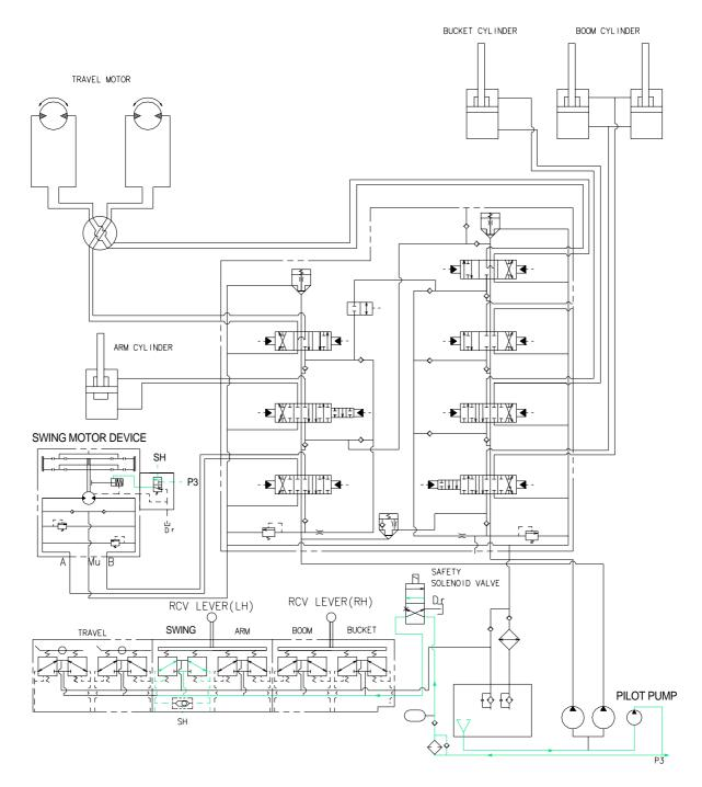
When the swing control lever is tilted, the pilot oil go to SH port of shuttle valve, this pressure move spool so, discharged oil from pilot pump go to P<sub>3</sub> port.
