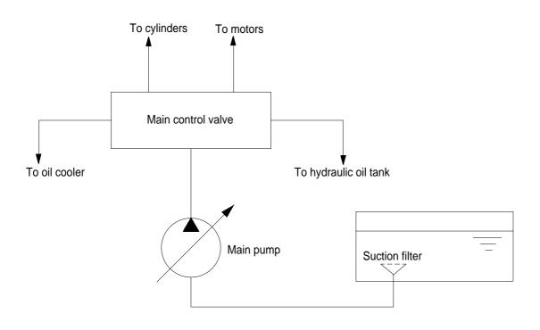
The pump receive oil from the hydraulic tank through a suction filter. The discharged oil from the pump flows into the control valve and goes out the tank ports.
