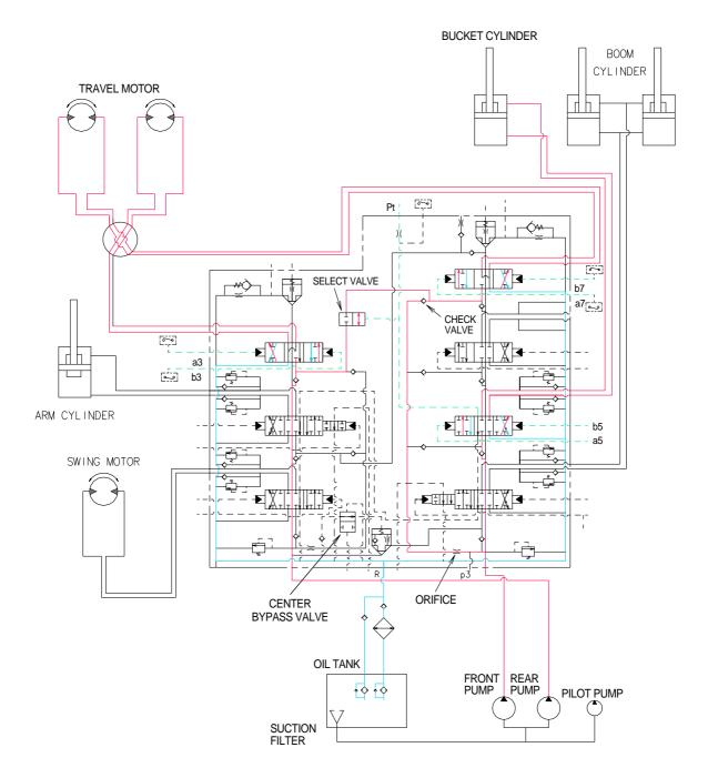
When the bucket and travel (R),(L) functions are operated, the bucket and travel (R),(L) spools and the select valve changed. The oil flows from rear pump through the travel (R),(L) section of the control valve to right and left travel motor and the machine travelling.
