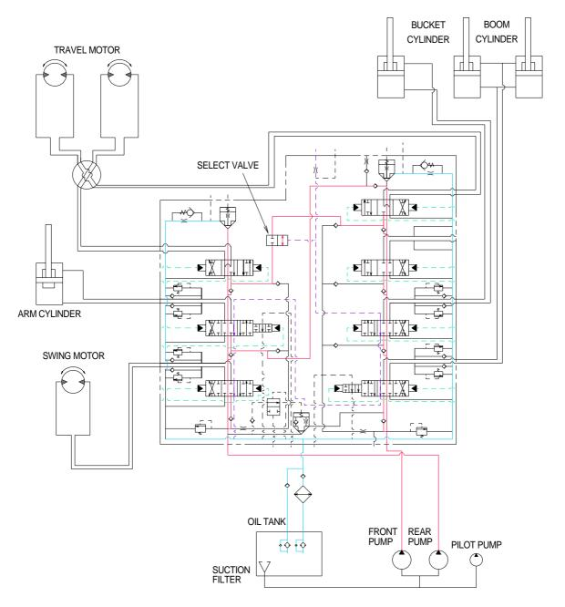
In case operation, the oil flows from both main pumps through the neutral oil passage, bypass oil passage and confluence oil passage. Then the oil is supplied to each actuator and function them. Check valves and orifices are provided with on these flow passage. These control the oil flows from the pump corresponding to the each actuator's state of functioning and smooth the combined operation.
