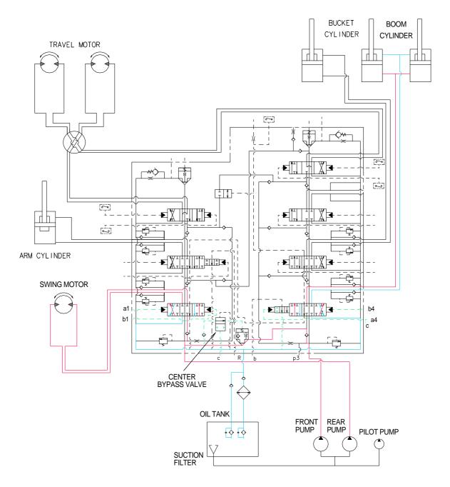
When the swing and boom functions are operated, simultaneously the swing spool and boom spools changed. The oil flows from the front pump through boom section of the control valve to boom cylinders and the boom functions.
