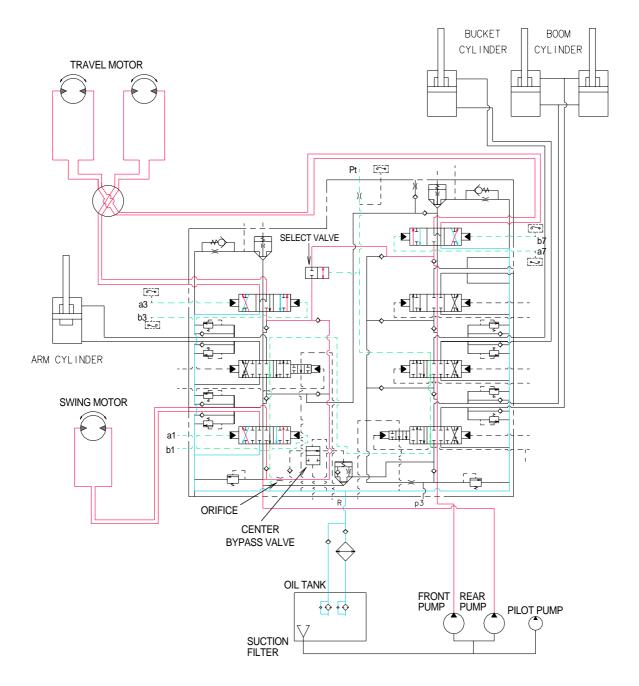
When the swing and right and left travel functions are operated, the swing and travel(R),(L) spools and the select valve changed. The oil flows from front pump through the travel (R),(L) section of the control valve to the right and left travel motor.
