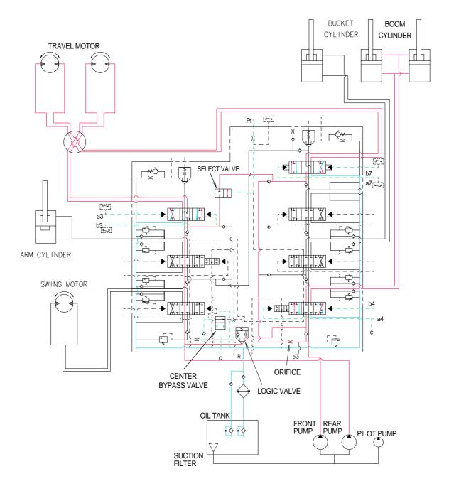
When the boom and travel (R) (L) functions are operated, the boom and travel (R),(L) spools and the select valve changed. The oil flows from front pump through the travel (R),(L)section of the control valve to the right and left travel motor.
