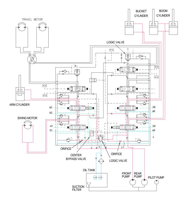
When the swing, boom, arm and bucket functions are operated, the each spools of the control valve changed.
