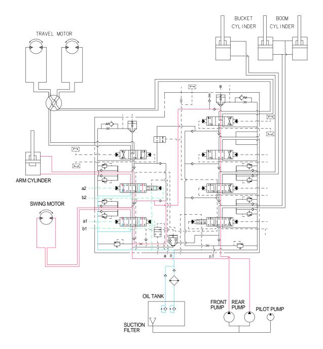
When the swing and arm functions are operated, simultaneously the swing and arm spools changed. The oil flows from the rear pump through arm and swing section of the control valve to arm cylinder and swing motor, and the arm and swing function.
