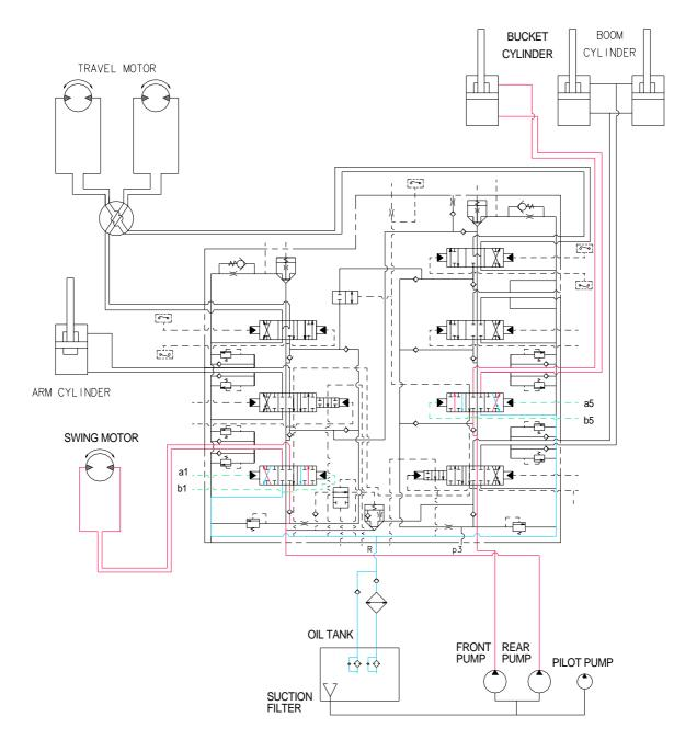
When the swing and bucket functions are operated, the swing and bucket spools changed. The oil flows front pump through the bucket section of the right control valve to the bucket cylinder and the bucket function. The oil flows from rear pump through swing section of the left control valve to the swing motor and swing the superstructure.
