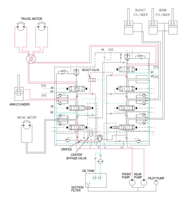
When the arm and travel (R) (L) functions are operated, the arm and travel (R),(L) spools and the select valve changed. The oil flows from front pump through the travel (R),(L) section of the control valve to the right and left travel motor.
