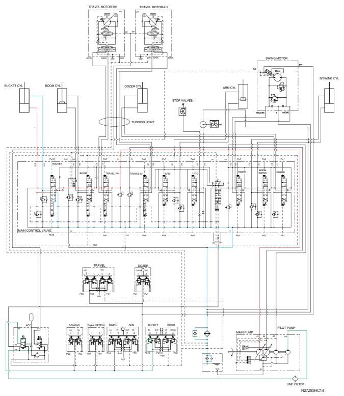
When the right control lever is pulled left, the bucket spool in the main control valve is moved to the roll in position by the pilot oil pressure from the remote control valve.
