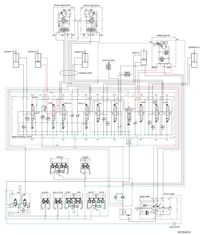
When the swing and boom functions are operated, simultaneously the swing spool and boom spools in the main control valve are moved to the functional position by the pilot oil pressure from the remote control valve.
