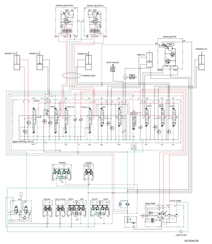
When the bucket and travel functions are operated, simultaneously the bucket spool and travel spools in the main control valve are moved to the functional position by the pilot oil pressure from the remote control valve, and the travel selector spool is pushed to the up by the oil pressure from pilot pump. The oil from the A1 and A2 pumps flows into the travel motors.
