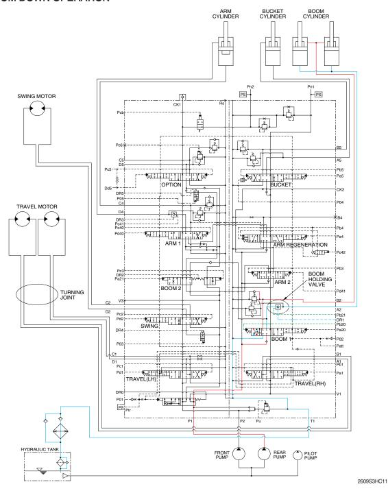
When the RH control lever is pushed forward, the boom spools in the main control valve are moved to the down position by the pilot oil pressure from the remote control valve.
