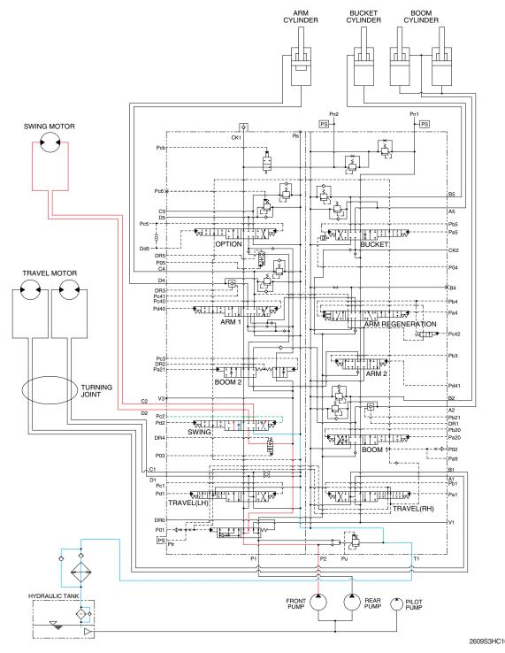
When the LH control lever is manually placed in the left (right) swing position. Then the oil flows from A1 pump through the swing section of the main control valve to swing motor to left (right) swing the superstructure. The return oil flows from swing motor through the swing section of the main control valve returned to the tank.
