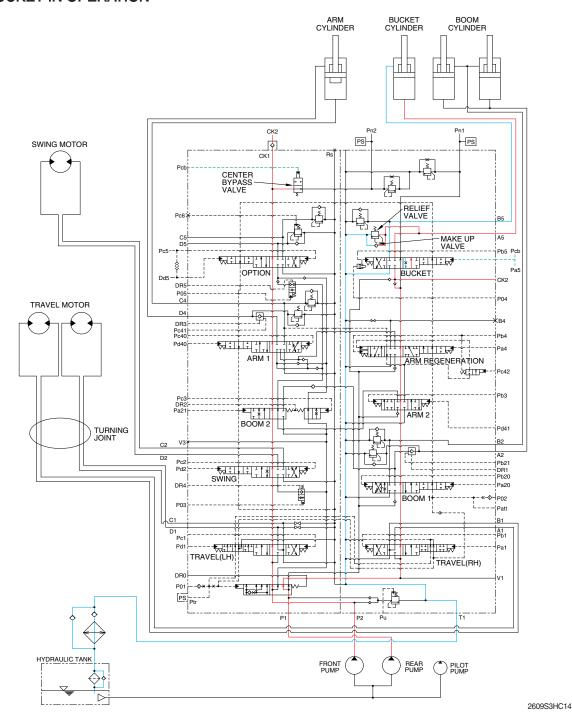
When the RH control lever is manually placed in the bucket roll in position. Then the oil flows from pilot pump through the pilot valve to bucket section of the main control valve. Here the spool position is moved to bucket roll in position.
