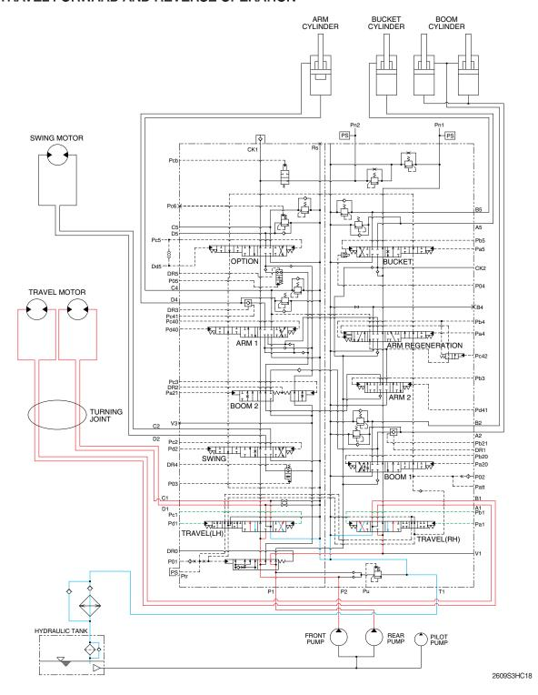
When the right and left travel levers are manually placed to the forward or reverse position, the oil flows from pilot pump through the pilot valve to travel sections of the main control valve.
