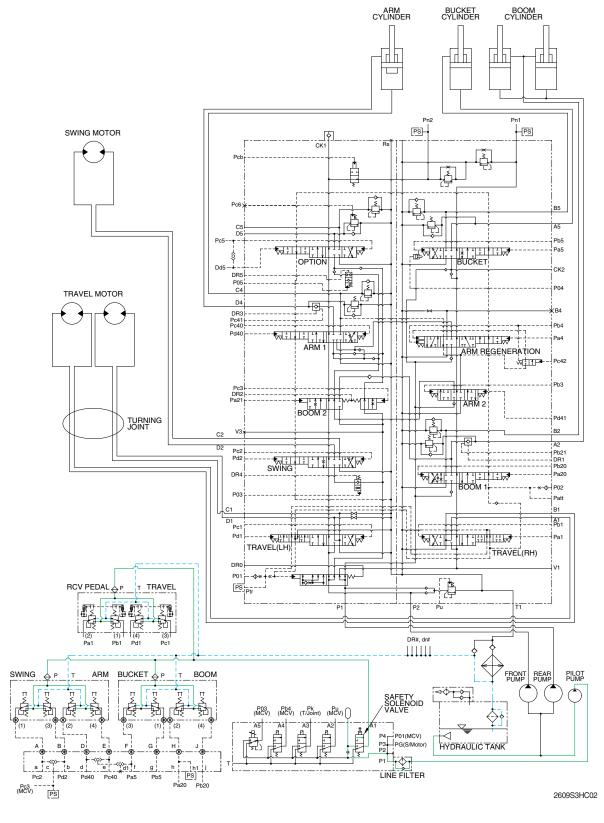
The pilot pump receive oil from the hydraulic tank. The discharged oil from the pilot pump flows to the safety solenoid valve through the line filter. The oil is filtered by the line filter. The pilot relief valve is provided in the pilot pump for limiting the pilot circuit pressure.
