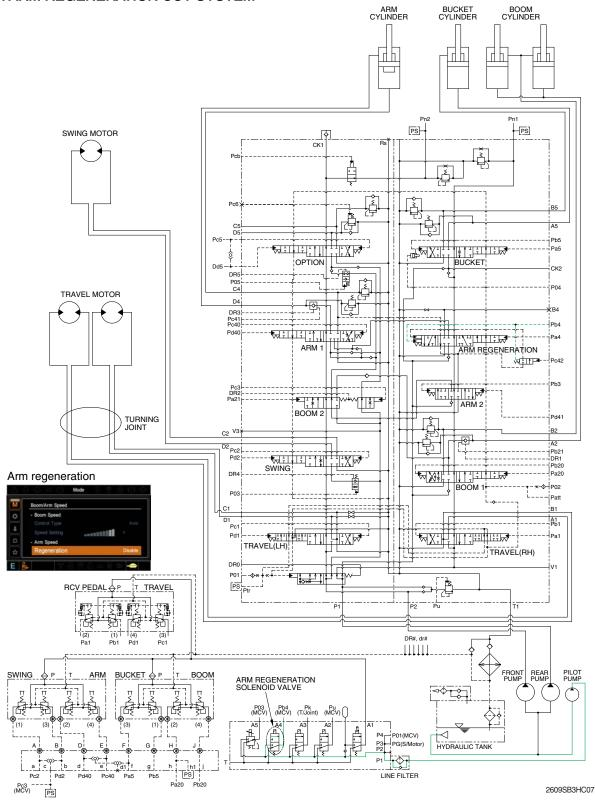
When the arm regeneration is selected to disable on the cluster, the arm regeneration solenoid valve is activated. The pilot oil from pilot pump flow into **Pb4** port in main control valve through solenoid valve and the arm regeneration spool is shifted to right.
