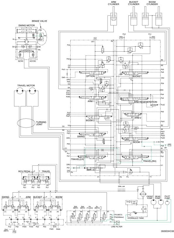
When one of the RCV lever (except travel lever) is tilted, the pilot oil flows into SH port through main control valve.
