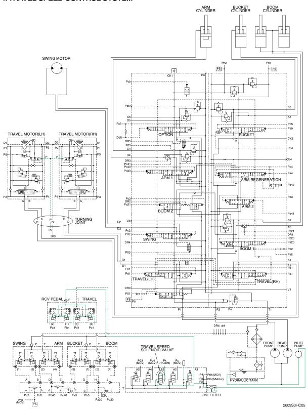
When the travel speed solenoid valve was placed in the Hi position, the pressure oil from pilot pump through line filter flows to port **P** of travel speed change over valve, and the control piston is pushed up, thus minimizing the displacement.
