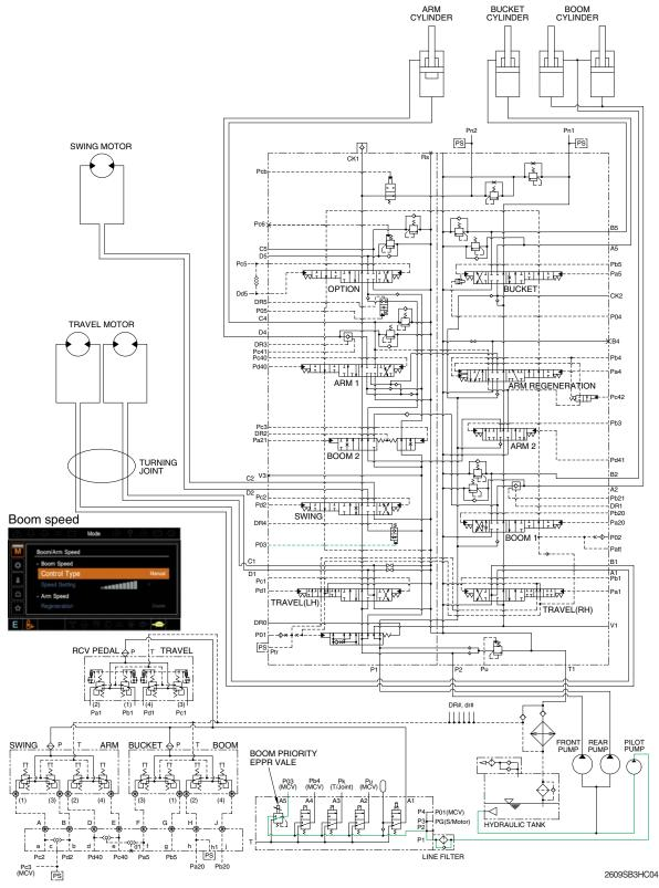
When carrying out the combined operation of swing and boom up, the boom up operating speed is lowered then normal operation.
