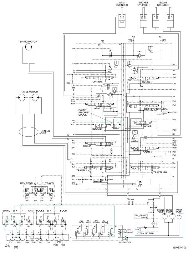
When carrying out the combined operation of swing and arm of the left control valve, the swing speed can be lowered than operating speed of arm.
