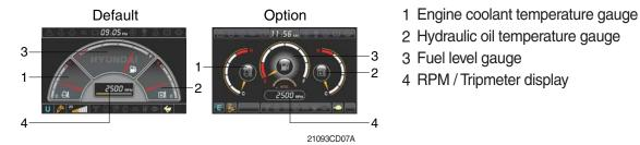
\* Operation screen type can be set by the screen type menu of the display. Refer to page 5-60 for details.
