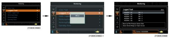
• The logged faults of the MCU can be checked by this menu.
