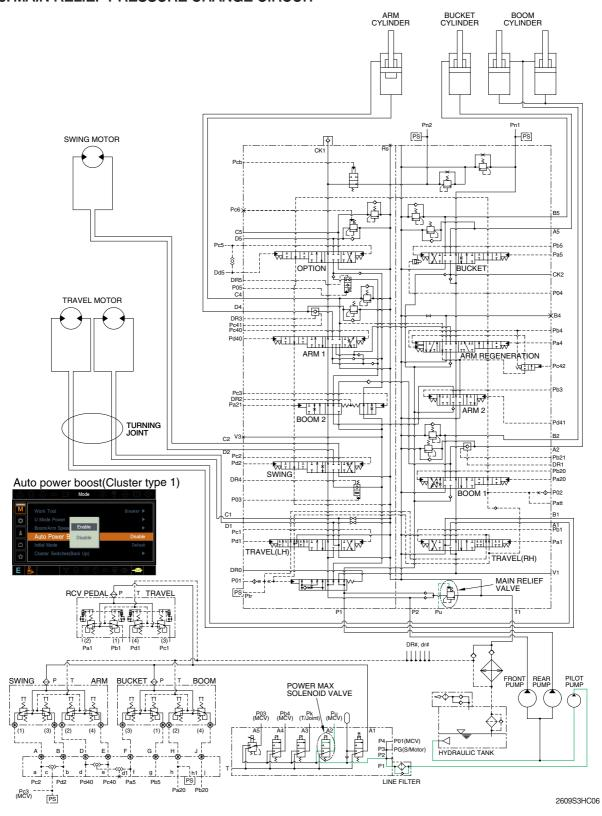
When the power max switch on the left control lever is pushed ON, the power max solenoid valve is actuated, the discharged oil from the pilot pump into Pu port of the main relief valve of main control valve; Then the setting pressure of the main control valve is raises from 350 kgf/cm² to 380 kgf/cm² for increasing the digging power. And even when press continuously, it is canceled after 8 seconds. When the auto power function is selected to enable on the cluster, the pressure of the main relief
