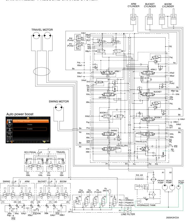
When the power boost switch on the left control lever is pushed ON, the power boost solenoid valve is actuated, the discharged oil from the pilot pump flows into **Pz** port of the main relief valve of main control valve; then the setting pressure of the main relief valve is raised from 350 kgf/cm² to 380 kgf/cm² for increasing the digging power.
