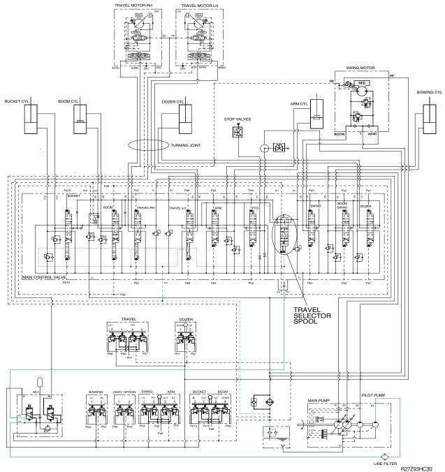
The oil from the A1, A2, A3 pump flows through the neutral oil passage, bypass oil passage and confluence oil passage in the main control valve. Then the oil goes to each actuator and operates them. Check valves and orifices are located on these oil passage in the main control valve. These control the oil from the main pumps so as to correspond to the operation of each actuator and smooth the combined operation.
