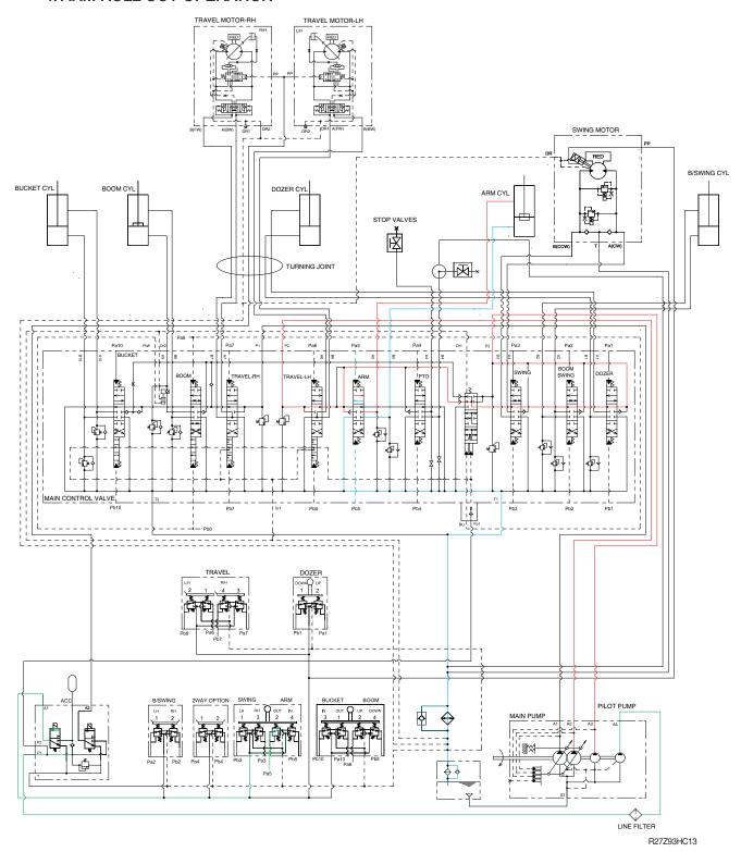
When the left control lever is pushed forward, the arm spool in the main control valve are moved to the roll out position by the pilot oil pressure from the remote control valve.
