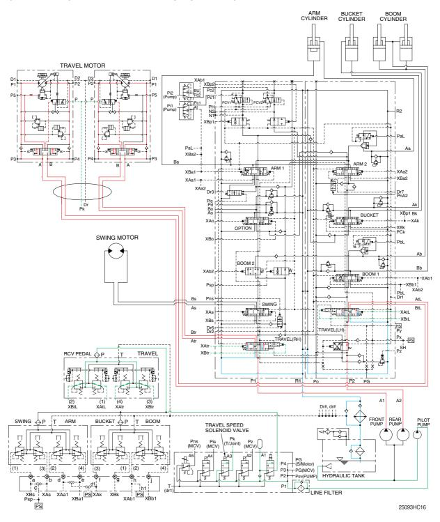
When the travel levers are pushed forward or reverse position, the travel spools in the main control valve are moved to the forward or reverse travel position by the pilot oil pressure from the remote control valve.
