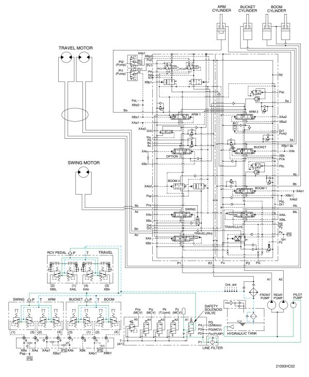
The pilot pump receive oil from the hydraulic tank. The discharged oil from the pilot pump flows to the safety solenoid valve through the line filter. The oil is filtered by the line filter. The pilot relief valve is provided in the pilot pump for limiting the pilot circuit pressure.
